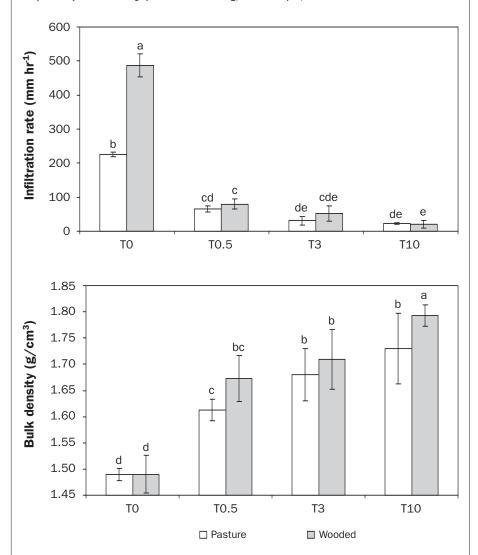
Table 4. Mean infiltration rate and bulk density result from tests conducted in the wheel ruts of a dump truck, backhoe and pickup after nine passes over a graded pasture. Means that were not significantly different were grouped with the same letter (n = 4 for each vehicle).
