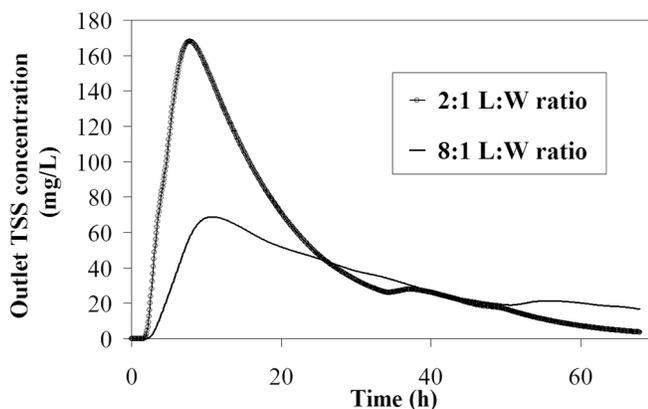
In agreement with the observed deposition patterns, the model indicated that most of the suspended solids did not travel beyond the forebay, as shown in Fig. 11, but some particles remaining in suspension continued through the outlet.
