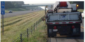
The first table below can be used to determine how much time it will take to spray 1 acre based on chosen nozzle spray width and ground speed. Use the second table to determine the distance in linear feet and lane miles to spray 1 acre based on nozzle spray width.
