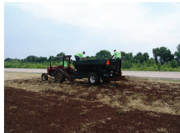
For larger areas, a manure spreader can be used to distribute the moist medium and seed mixture.
