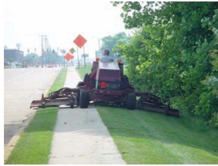
Various mowers are used depending on the desired cut width and maneuverability required.
