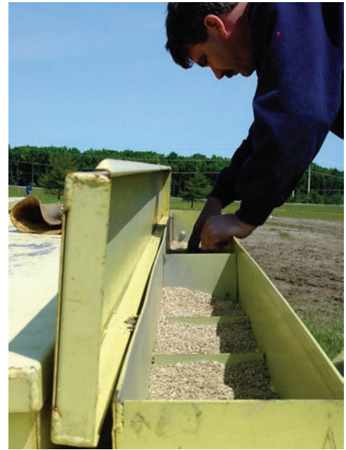
Seed boxes in a Truax drill separate fluffy seeds and small seeds to provide even distribution.
