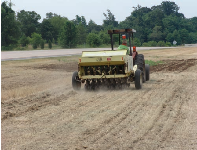
Capable of handling various size seeds, a Truax drill delivers seeds into a planting furrow, providing good seed/soil contact.
