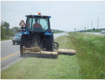
Various mowers are used depending on the desired cut width and maneuverability required.
