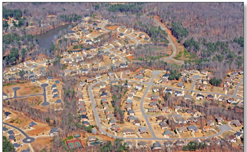
Figure 9. Urban sprawl in the west Atlanta Metropolitan Area, Douglas County, Georgia. Low-density large-lot residential development creates more impervious cover through more driveways, streets, and sidewalks than integrating small lots with public parks and natural areas.
