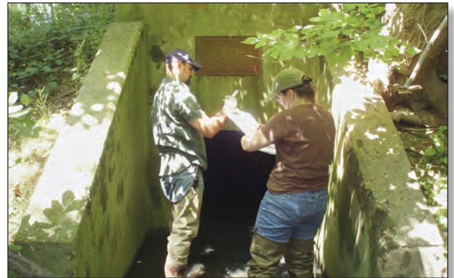
Figure 38. Team conducting dry weather outfall sampling for illicit discharges in the Jones Falls watershed in Baltimore, Maryland. Photograph from Center for Watershed Protection.
