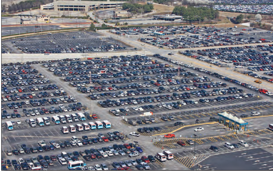
Figure 12. Impervious cover includes surfaces that do not allow rainwater to infiltrate, such as this parking lot at the Hartsfield-Jackson Atlanta International Airport. As impervious cover increases in a watershed, the condition of streams declines as a result of increased runoff volume and velocity and the introduction of various pollutants to the stream.
