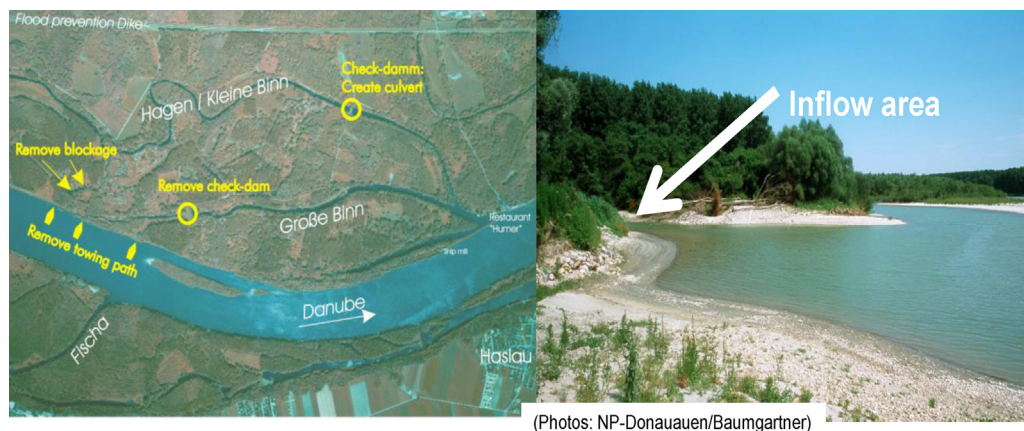
Fig. 5. Left picture: Satellite image of the restoration measures in the floodplain area of Orth. The "birds eye view" clearly shows some old anabranches and meanders and the measures implemented. – © NationalparkDonau-Auen and OeBF group. Right: Photograph of the inflow area in Orth. Right side of the photograph the river main channel can be seen. – © NationalparkDonau-Auen/Baumgartner.
