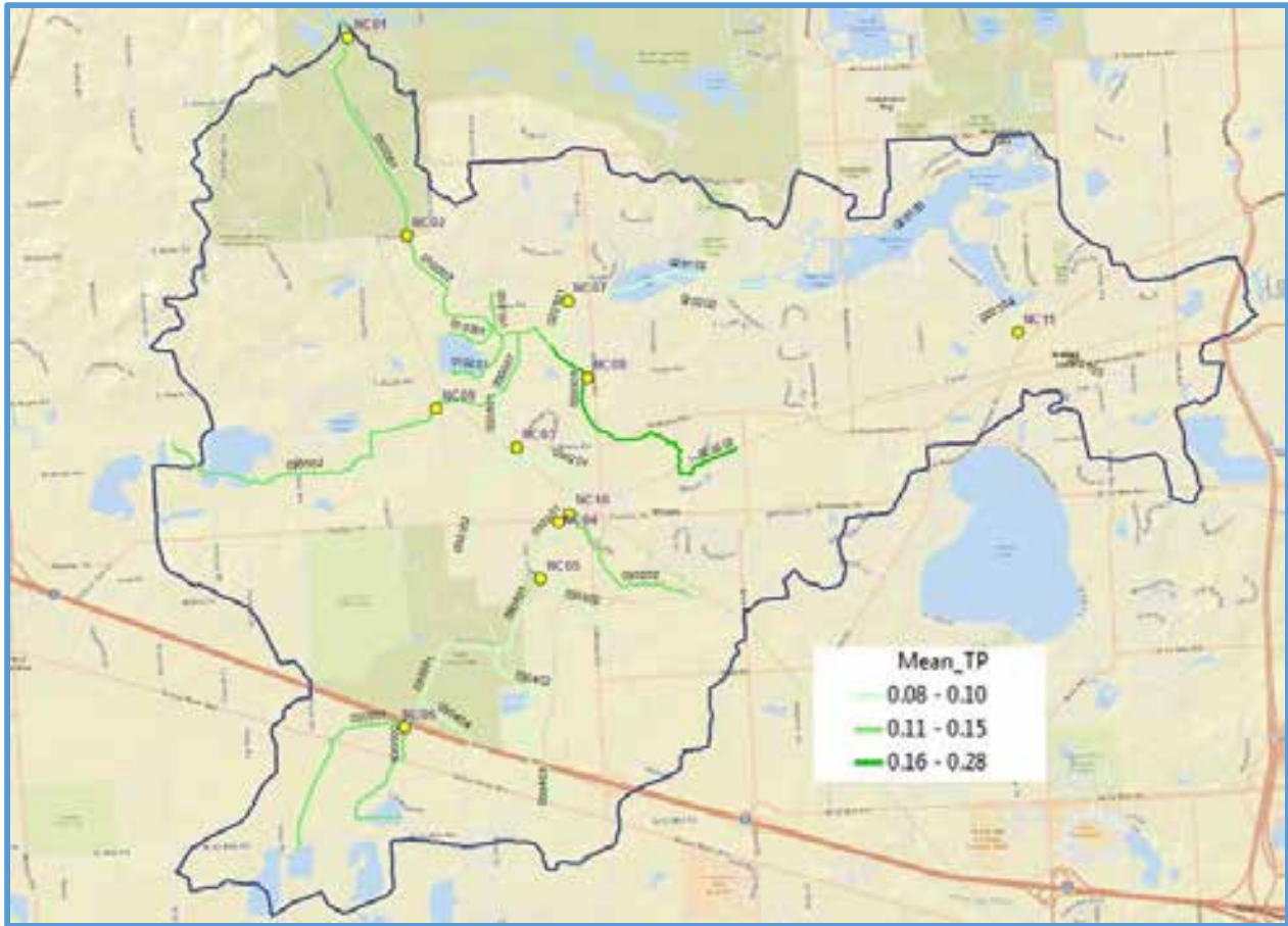
Figure 13: Norton Creek watershed showing stream reaches with corresponding total phosphorus concentrations in mean mg/l.
