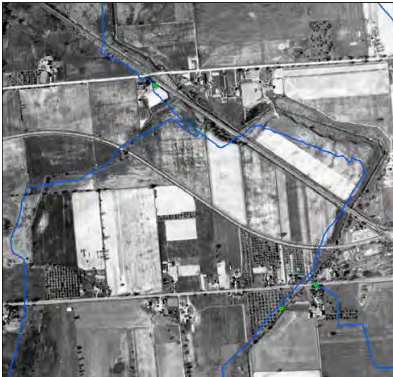
Figure 9: Section of current Norton Creek stream network (between Pontiac Trail and Maple Road) shown on an aerial photo from 1949. Note that the photo is not orthorectified, so the channels do not exactly match. However, current channel shape matches almost identically to 1949.
