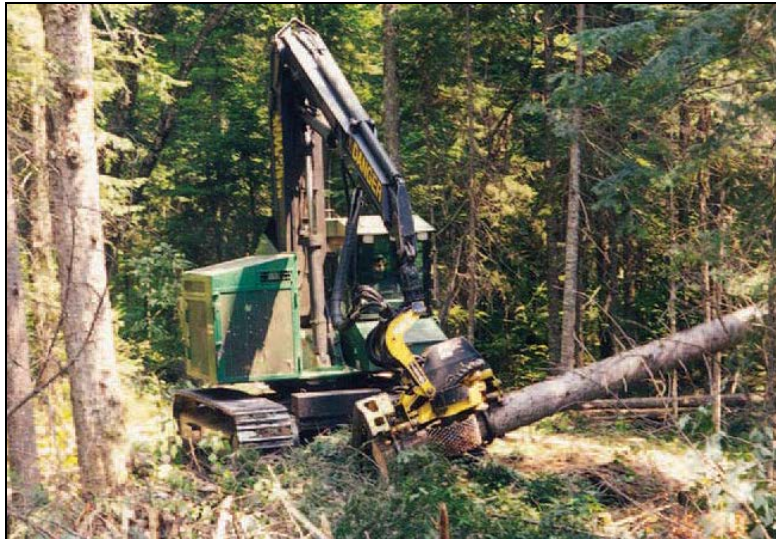
Figure 3. A Tracked Harvester with Extendable Boom.
