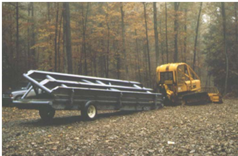
Figure 19. A Portable Folding Metal Bridge.
