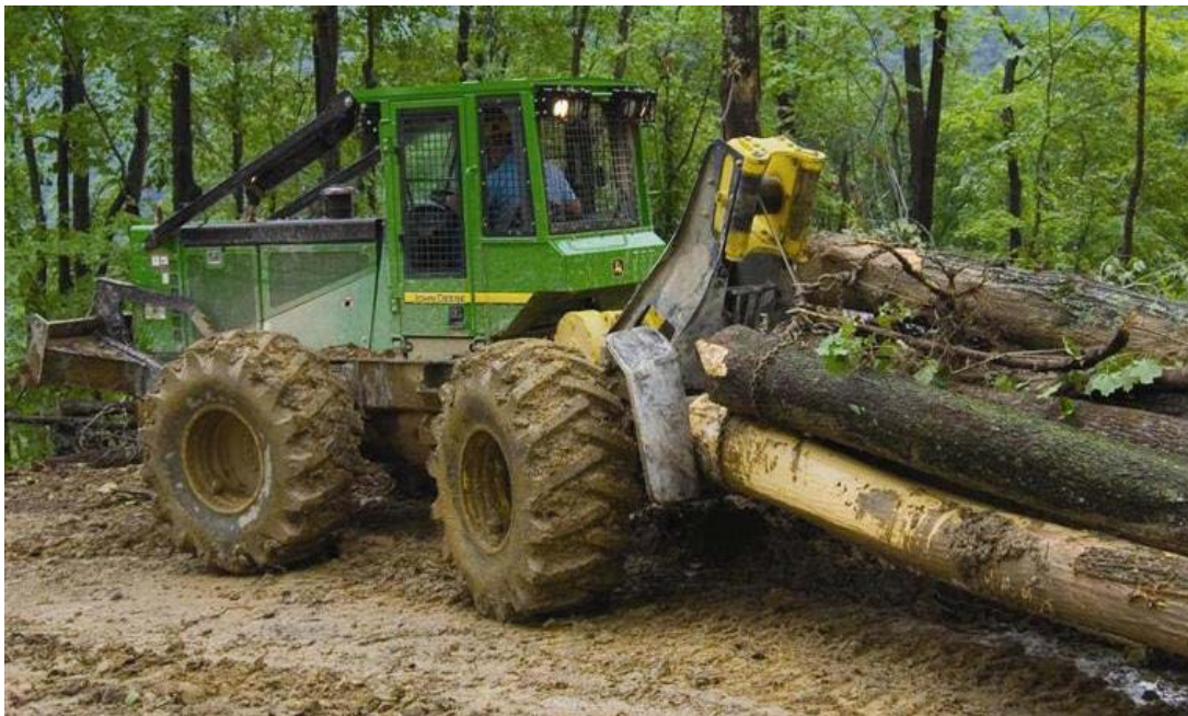
Figure 25. John Deere 640H Cable Skidder.
