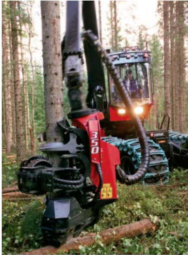
Figure 24. Cut-to-Length Harvester-Processor with Tracked Wheels.
