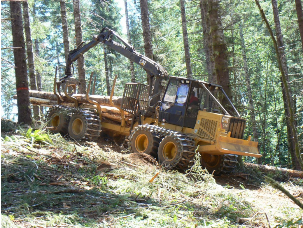
Figure 27. Caterpillar 574 Forwarder with Tracked Wheels.
