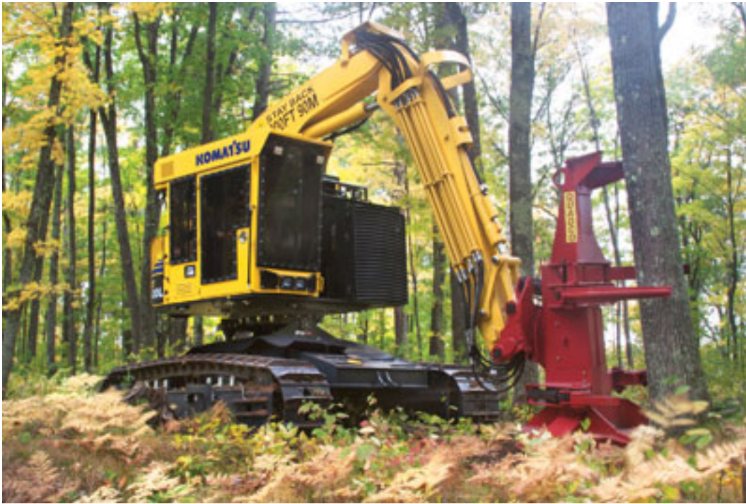
Figure 22. Tracked Komatsu XT Series Feller-Buncher.
