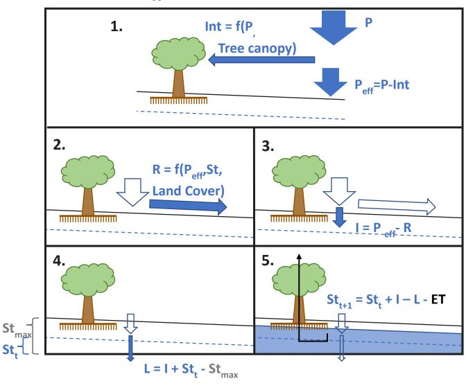
**Figure 2.** Conceptual model of step-wise calculations used in the water yield model. Box 1 corresponds to equations 2 and 3, and Boxes 2 to 5 correspond to equations 4 to 7, respectively.
