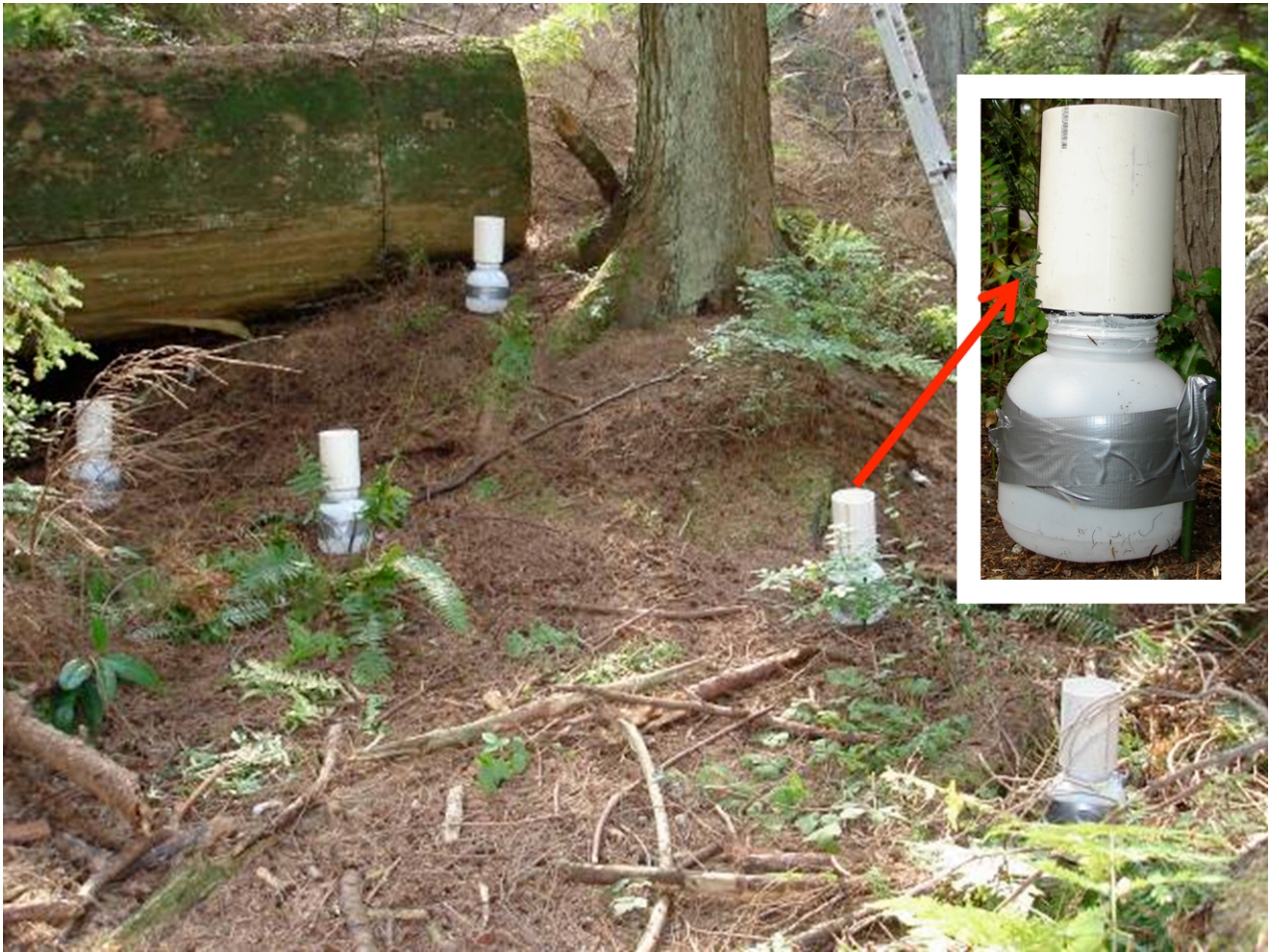
Figure 2.8: Random distribution of point throughfall collectors under a Douglas-fir (Tag# 6) in Lighthouse Park
