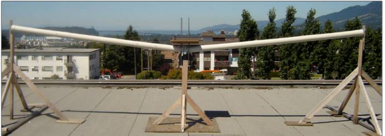
Figure 2.7: Example of reference rainfall gauge installed on the rooftop of North Vancouver's City Hall to measure gross precipitation (above canopy rainfall).
