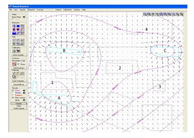
Figure 2: Flowlines with potentials (arrows indicate flow direction; longer arrows indicate higher flow velocity). This situation is considering infiltration from three sources. Numbers are buildings while letters are infiltration areas.
