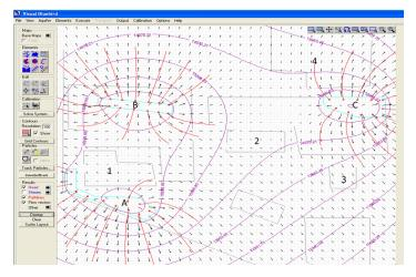
Figure 4 shows maximum water droplet movement over a one day period and shows approximately 50 m of travel.
