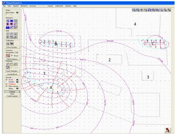
Figure 5: Estimate of underdrain impact on surrounding structures.
