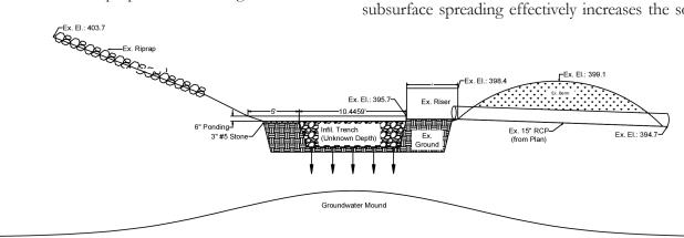
Figure 1: An example groundwater mound beneath an infiltration trench.
