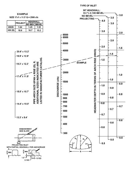
BUREAU OF PUBLIC ROADS OFFICE OF R&D JULY 1966 HEADWATER DEPTH FOR INLET CONTROL STRUCTURAL PLATE PIPE-ARCH CULVERTS 31 in. RADIUS CORNER PLATE PROJECTING OR HEADWALL INLET HEADWALL WITH OR WITHOUT EDGE BEVEL
