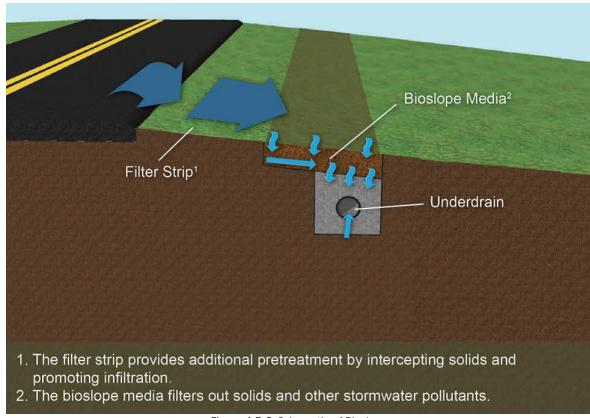
Figure 4.3-2 Schematic of Bioslope (Source: GDOT Drainage Manual, 2014)
