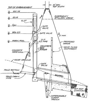
Figure 3.4.2-9 Schematic of Combination Outlet Structure
