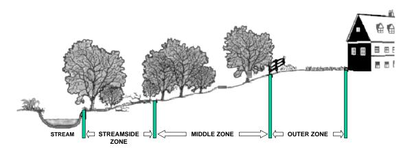
Figure 2.3.2-4 Three-Zone Stream Buffer System
