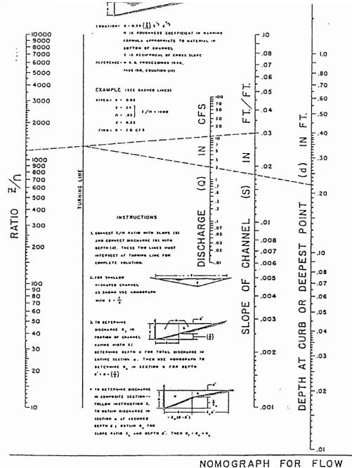
NOMOGRAPH FOR FLOW IN TRIANGULAR CHANNELS
