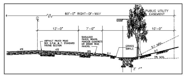
Figure 5.1-1 Alternate Roadway Section without Gutters
