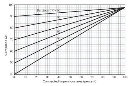
Figure 3.1.5-3 Composite CN with Connected Impervious Areas (Source: NRCS TR-55, NEH630, 2004)
