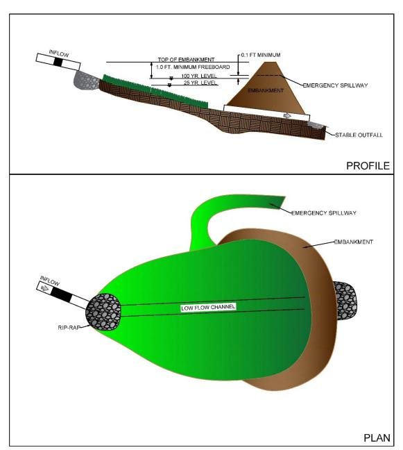
Figure 4.5-1 Schematic of Dry Detention Basin
