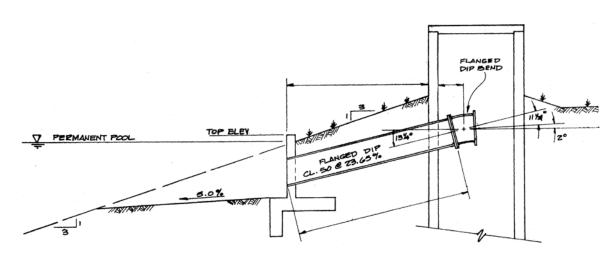
Figure 3.4.5-1 Reverse Slope Pipe Outlet
