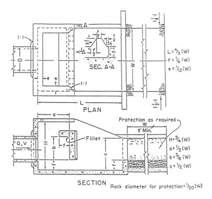
Figure 5.5-11 Schematic of Baffled Outlet
