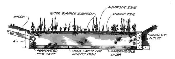
Figure 4.27-1 Schematic of Submerged Gravel Wetland System
