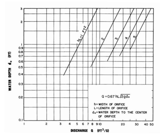
Figure 5.2-11 Curb-Opening Inlet Orifice Capacity for Inclined and Vertical Orifice Throats
