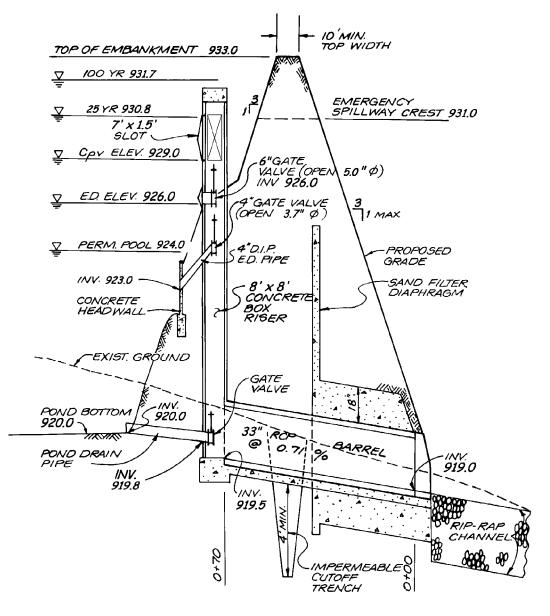
Figure 8. Profile of Principle Spillway
