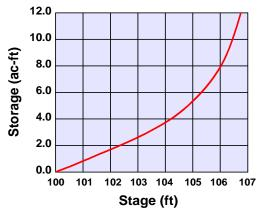
Figure 3.3.1-3 Stage-Storage Curve
