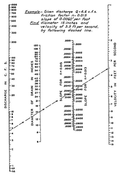
Figure 5.2-14 Nomograph for Computing Required Size of Circular Drain,
