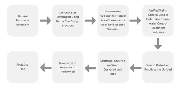
Figure 2.2.5-2 Typical Stormwater Management System Design Process
