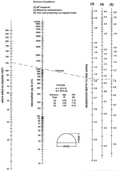
HEADWATER DEPTH FOR C.M. ARCH CULVERTS 0.3 ≤ RISE/SPAN < 0.4 WITH INLET CONTROL
