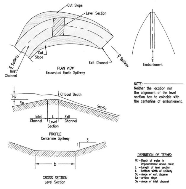
Figure 3.4.7-1 Emergency Spillway
