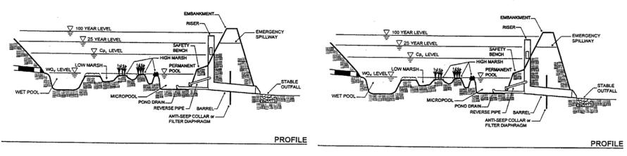
Figure 4.26-4 Schematic of Pond/Wetland System
