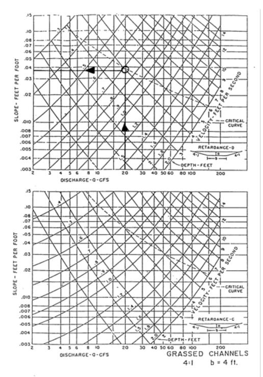
**Figure 5.4-15** Example Nomograph #5 (Source: FHWA)
