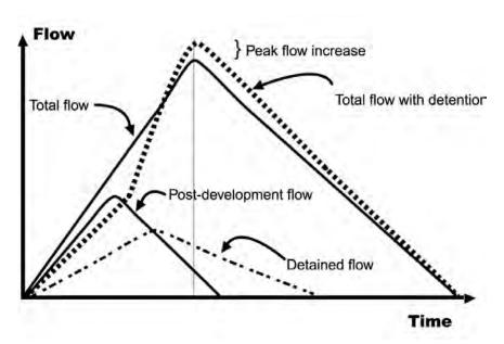
Figure 3.1.9-1 Detention Timing Example
