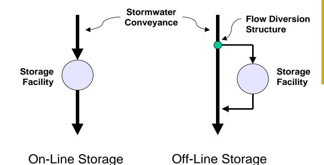
Figure 3.3.1-2 On-Line versus Off-Line Storage
