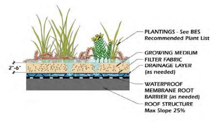
Figure 4.11-3: Extensive Green Roof System (Source: City of Portland, OR, 2004)
