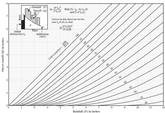
Figure 3.1.5-2 NRCS TR-55 Solution of the Runoff Equation (Source: NRCS TR-55, NEH630, 2004)
