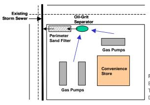
Figure 4.1.6-4 Example Treatment Train - Commercial Development
