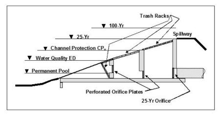
Figure 3.4.2-4 Schematic of Orifice Plate Outlet Structure
