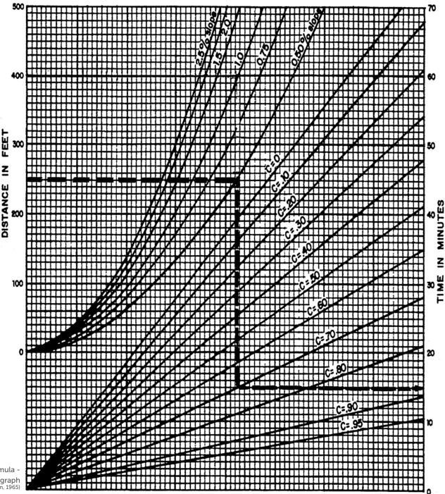
Figure 3.1.4-1 Rational Formula Overland Time of Flow Nomograph
