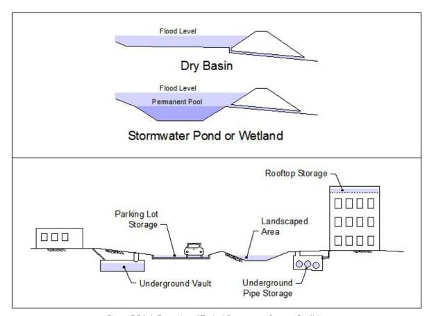
Figure 3.3.1-1 Examples of Typical Stormwater Storage Facilities
