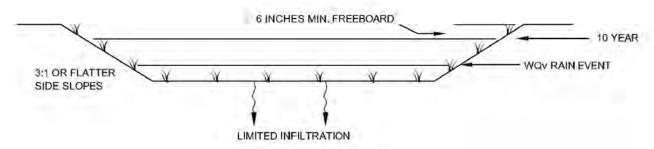
Figure 4.29-1 Typical Vegetated Filter Strip
