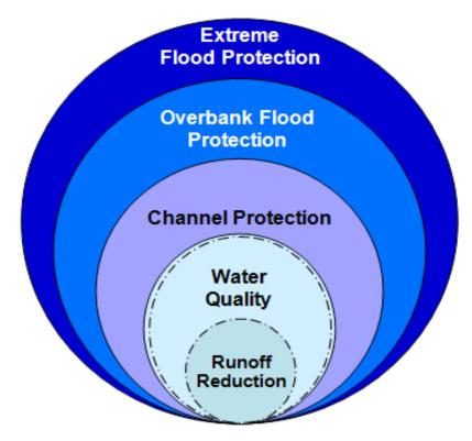
Figure 2.2.3-1 Representation of the Unified Stormwater Sizing Criteria
