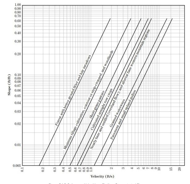
Figure 3.1.5-5 Average Velocities - Shallow Concentrated Flow (Source: NRCS TR-55, NEH630, 2004)
