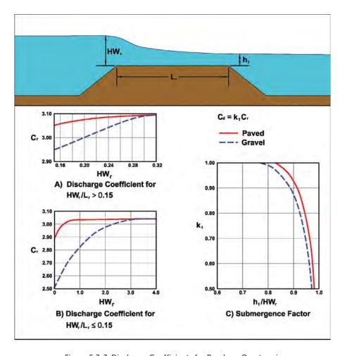
Figure 5.3-3 Discharge Coefficients for Roadway Overtopping
