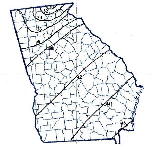
Figure 3.1.8-1 Average Annual Free Water Surface Evaporation (in inches) (Source: NOAA, 1982)
