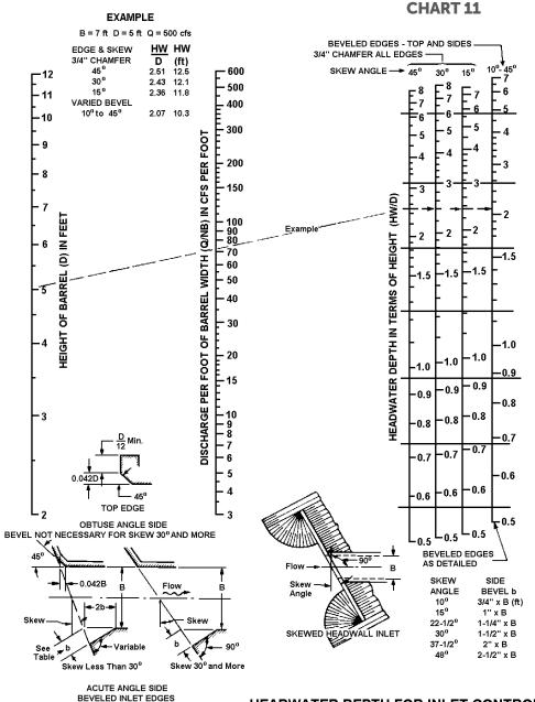
HEADWATER DEPTH FOR INLET CONTROL SINGLE BARREL BOX CULVERTS SKEWED HEADWALLS
