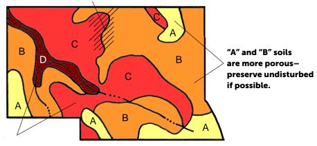
"C" and "D" soils should be used for impervious surface and buildings.
