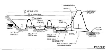
Figure 4.25-5 Schematic of Multiple Pond System
