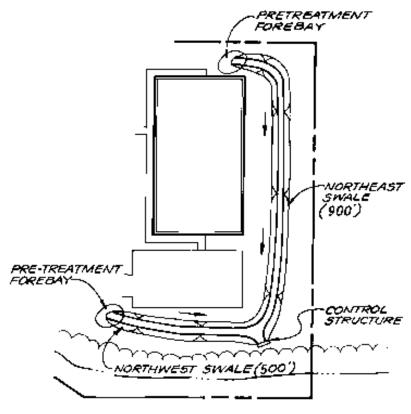
Figure 2. Enhanced Dry Swale Site Plan
