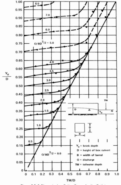
Figure 5.5-6 Dimensionless Rating Curves for the Outlets of Rectangular Culverts on Horizontal and Mild Slopes
