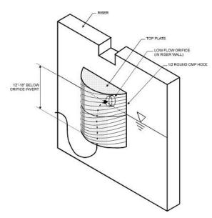
Figure 3.4.5-3 Half-Round CMP Orifice Hood
