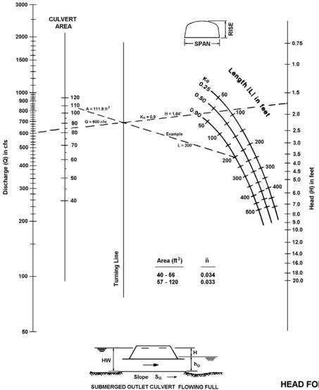
Nomographs adapted from material furnished by Kaiser Aluminum and Chemical Corporation. Duplication of this nomograph may distort scale. HEAD FOR
