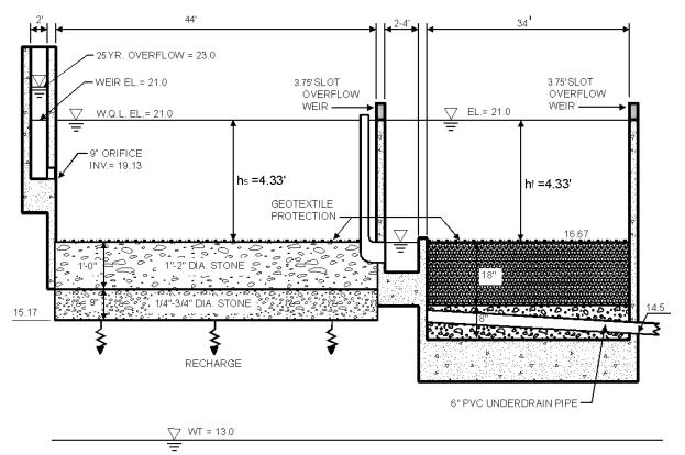
Figure 6. Plan and Profile of Surface Sand Filter
