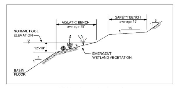
Figure 4.25-6 Typical Stormwater Pond Geometry Criteria
