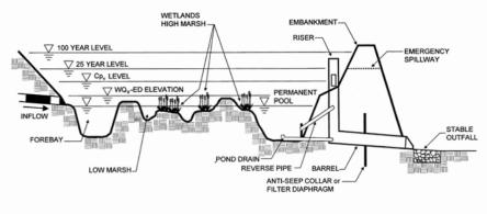
Figure 4.26-2 Schematic of Shallow Wetland
