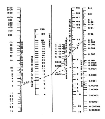
Figure 5.2-13 Nomograph for Solution of Manning's Formula for
