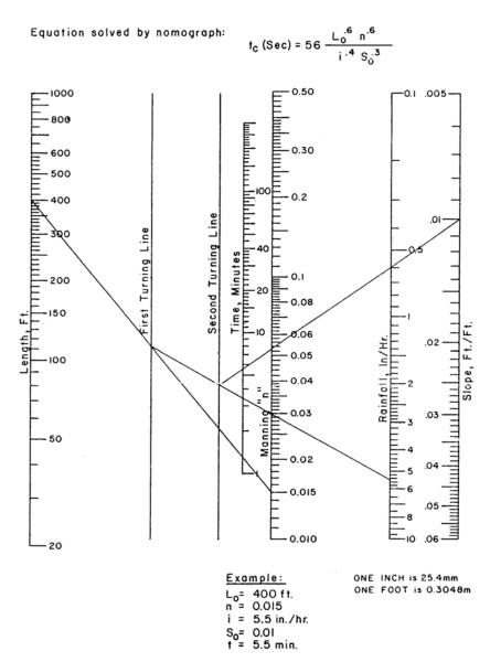
Figure 3.1.4-3 Kinematic Wave Nomograph (Source: Manual For Erosion And Sediment Control In Georgia)
