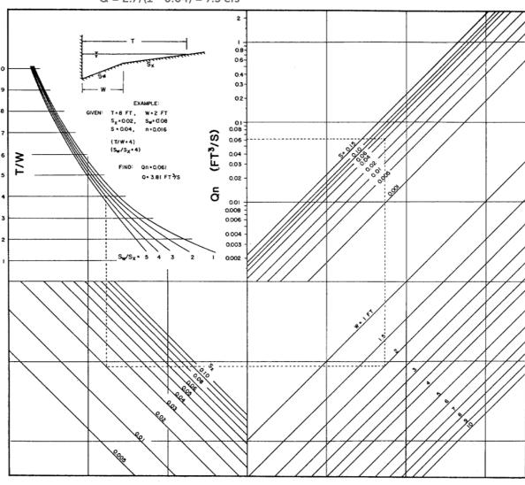
Figure 5.2-3 Flow in Composite Gutter Sections (Source: AASHTO Model Drainage Manual, 1991)
