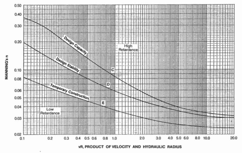
**Figure 5.4-1** Manning's n Values for Vegetated Channels (Source: USDA, TP-61, 1947)
