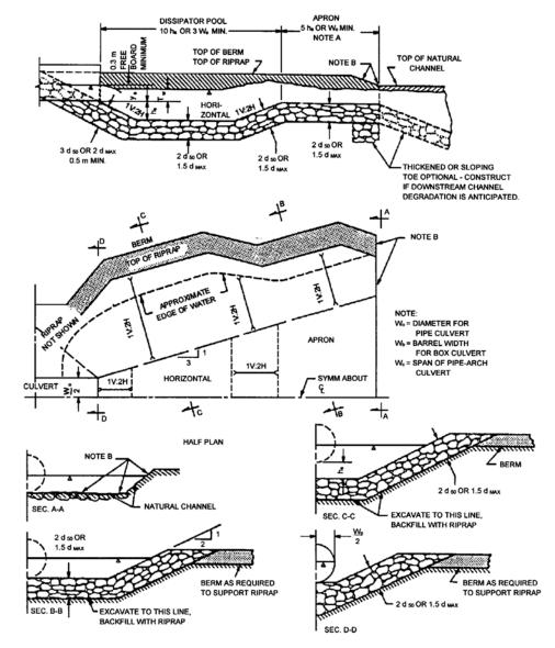
NOTE A - IF EXIT VELOCITY OF BASIN IS SPECIFIED, EXTEND BASIN AS REQUIRED TO OBTAIN SUFFICIENT CROSS-SECTIONAL AREA AT SECTION A-A SUCH THAT Q/(CROSS SECTION AREA AT SEC. A-A) = SPECIFIED EXIT VELOCITY.
