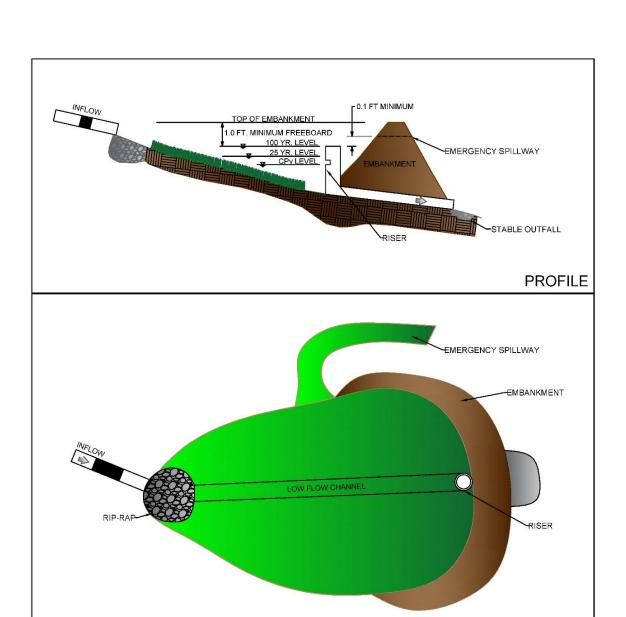
Figure 4.6-1 Schematic of dry ED Basin
