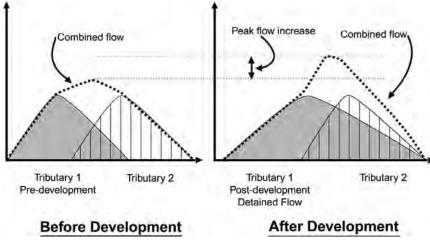
Figure 3.1.9-2 Effect of Increased Post-Development Runoff Volume with Detention on a Downstream Hydrograph
