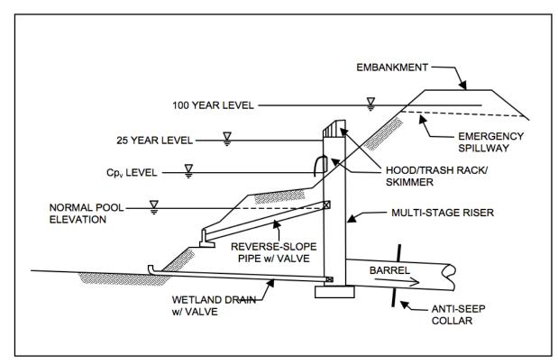
Figure 4.26-6 Typical Wetland Facility Outlet Structure
