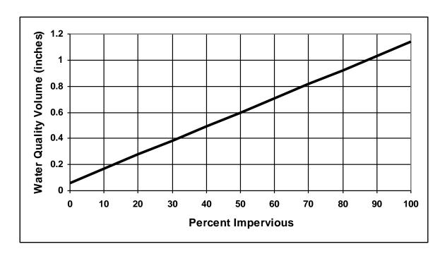
Figure 2.2.4-1 Water Quality Volume versus Percent Impervious Area
