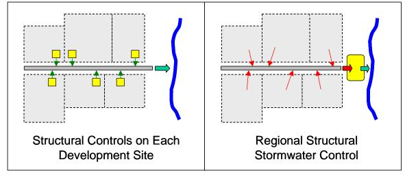
Figure 4.1.5-1 On-site versus Regional Stormwater Management
