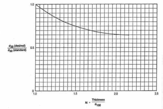
Figure 5.4-10 Riprap Lining Thickness Adjustment for  $d_{85}/d_{15} = 1.0$  to 2.3 (Source: Maynord, 1987)
