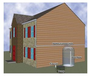
Figure 4.19-2: Major Components of a Rainwater
