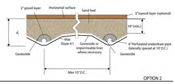
Figure 4.21-2 Typical Sand Filter Media Cross Sections
