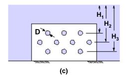
Figure 3.4.2-2 Orifice Definition
