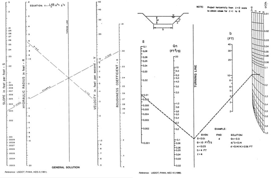
Figure 5.4-2 Nomograph for the Solution of Manning's Equation
