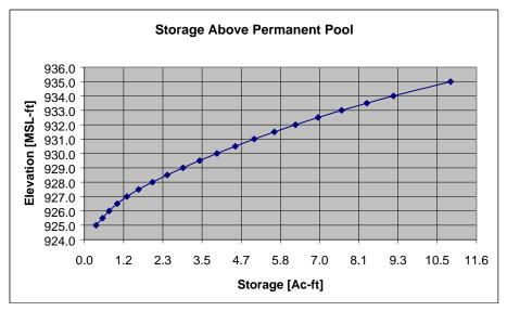
Figure 6. Storage-Elevation Table/ Curve
