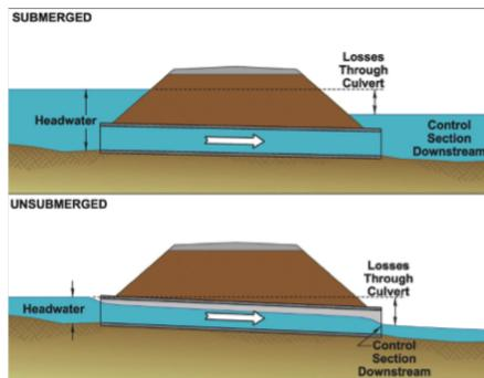
Figure 5.3-1(b) Typical Outlet Control Flow Conditions
