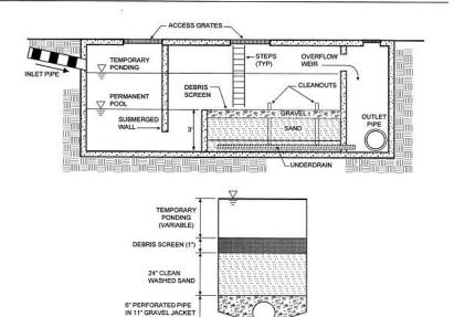
Figure 4.21-5 Schematic of Underground Sand Filter (Source: Center for Watershed Protection
