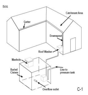
Figure 4.19-1: Rainwater Harvesting System (Source: Rupp, 1998)
