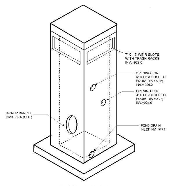
Figure 9. Schematic of Riser Detail
