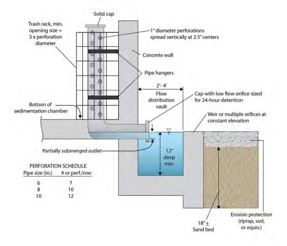
Figure 7. Perforated Stand Pipe Detail
