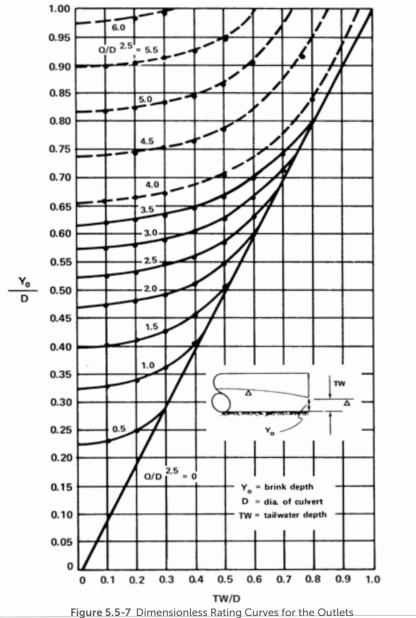
of Circular Culverts on Horizontal and Mild Slopes
