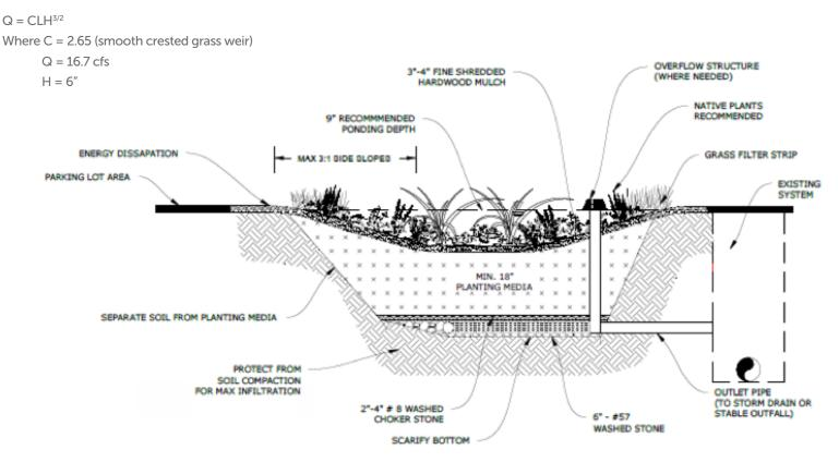
Figure 2. Typical Section of Bioretention Facility
