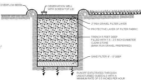
Figure 2. Infiltration Trench Cross Section
