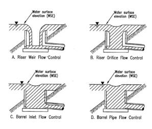
Figure 3.4.4-1 Riser Flow Diagrams
