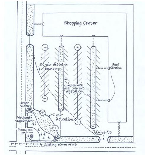
Figure 4.1.6-5 Example Treatment Train – Commercial Development (Source: NIPC, 2000)
