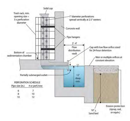
Figure 4.21-8 Surface Sand Filter Perforated Stand-Pipe (Source: GDOT Drainage Manual, 2014)
