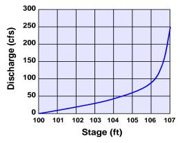
Figure 3.3.1-5 Stage-Discharge Curve
