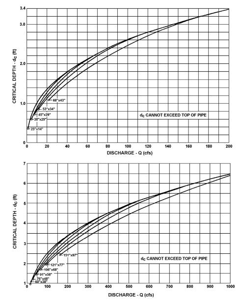
CRITICAL DEPTH OVAL CONCRETE PIPE LONG AXIS HORIZONTAL
