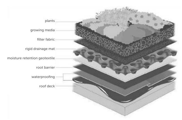
Figure 4.11-1: Components of a Green Roof System (Source: Carter et al., 2007)
