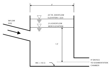
Figure 4. Flow Diversion Structure
