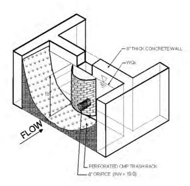
Figure 3 Control Structure at End of Swale
