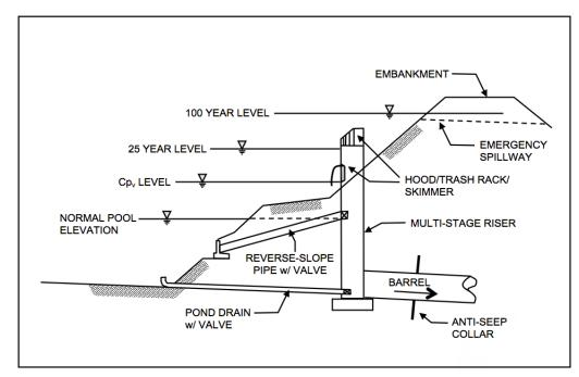
Figure 4.25-7 Typical Pond Outlet Structure
