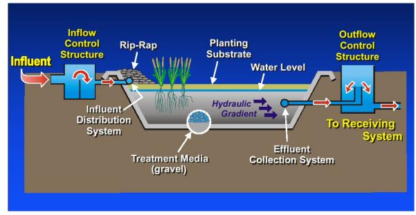
Figure 4.27-2 Schematic of Submerged Gravel Wetland System
