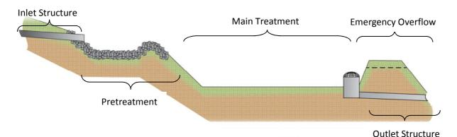
Figure 1 - Components of a BMP
