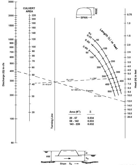
Nomographs adapted from material furnished by Kaiser Aluminum and Chemical Corporation. Duplication of this nomograph may distort scale. SUBMERGED OUTLET CULVERT FLOWING FULL
