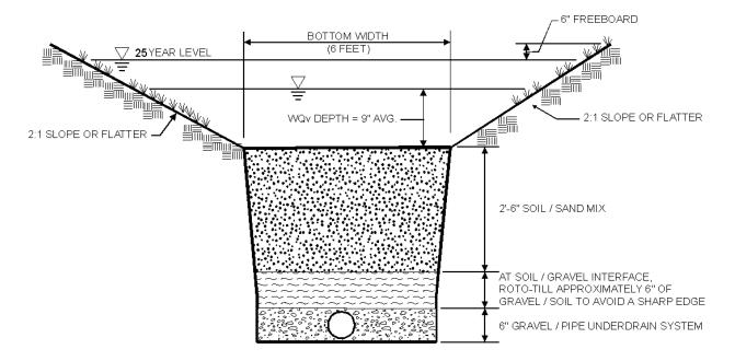
Figure 4 Trapezoidal Dry Swale Section
