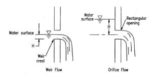
Figure 3.4.4-2 Weir and Orifice Flow (Source: VDCR, 1999)
