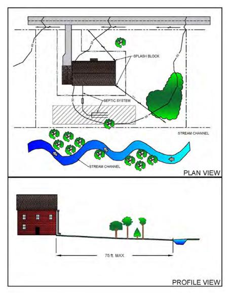
Figure 4.4-3 Schematic of Downspout Disconnect
