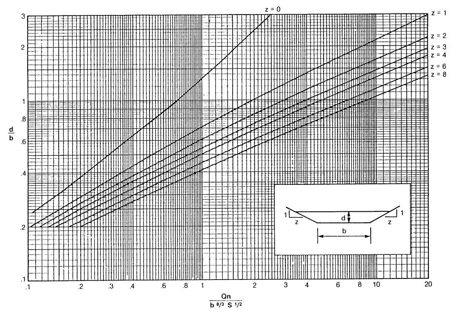
Figure 5.4-4 Trapezoidal Channel Capacity Chart
