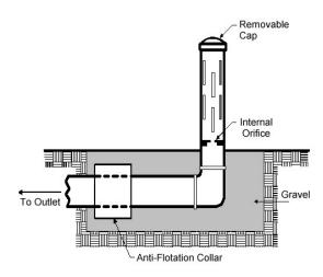
Figure 3.4.5-4 Internal Control for Orifice Protection
