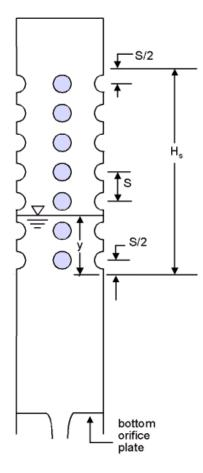
Figure 3.4.2-3 Perforated Riser
