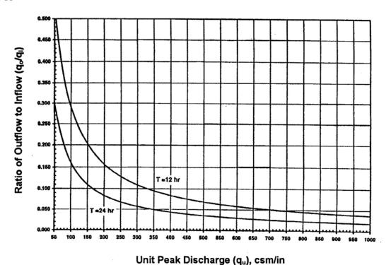
Figure 3.3.5-1 Detention Time vs. Discharge Ratios
