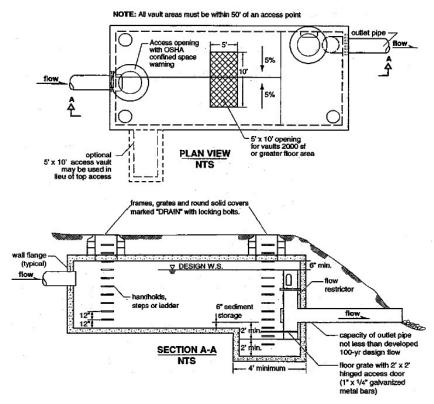
Figure 4.28-2 Example Underground Detention Tank System
