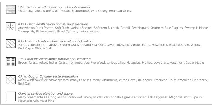
Figure D-5 Legend of Hydrologic Zones Around Stormwater Facilities
