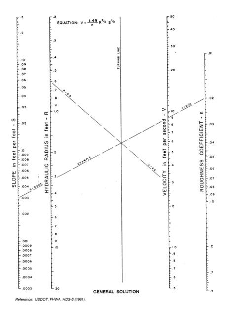
Figure 3.1.4-2 Manning's Equation Nomograph (Source: USDOT, FHWA, HDS-3 (1961))
