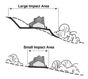
Figure 2.3.2-6 Flattening Steep Slopes for Building Sites Uses More Land Area Than Building on Flatter Slopes (Source: MPCA, 1989)
