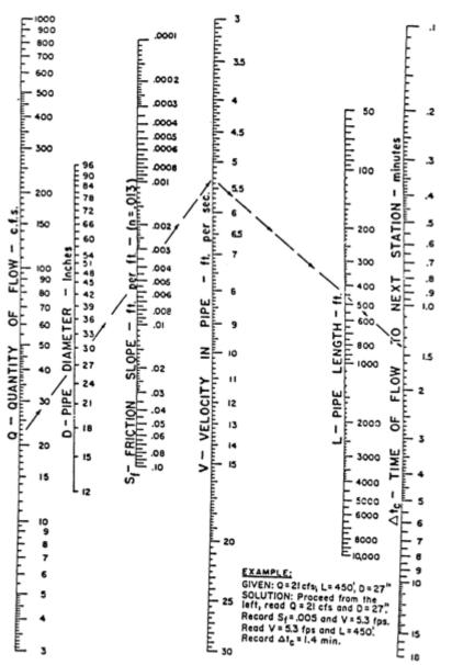
Figure 5.2-15 Concrete Pipe Flow Nomograph
