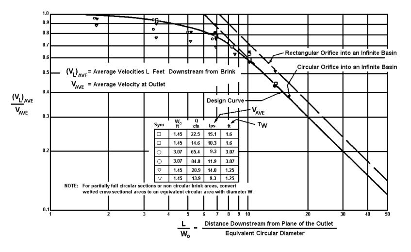
Figure 5.5-9 Distribution of Centerline Velocity for Flow from Submerged Outlets to Be Used for Predicting Channel Velocities Downstream from Culvert Outlet Where High Tailwater Prevails
