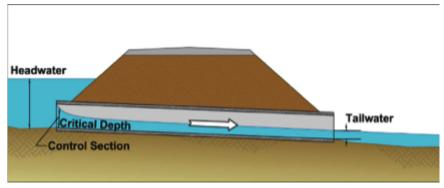
Figure 5.3-1(a) Typical Inlet Control Flow Section
