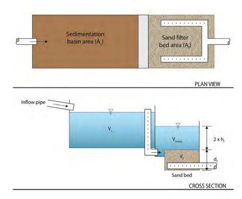
Figure 4.21-6 Surface Sand Filter Volumes Source: GDOT Drainage Manual, 2014
