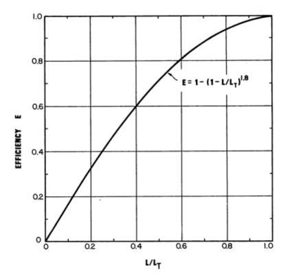
Figure 5.2-8 Curb-Opening and Slotted Drain Inlet Interception Efficiency
