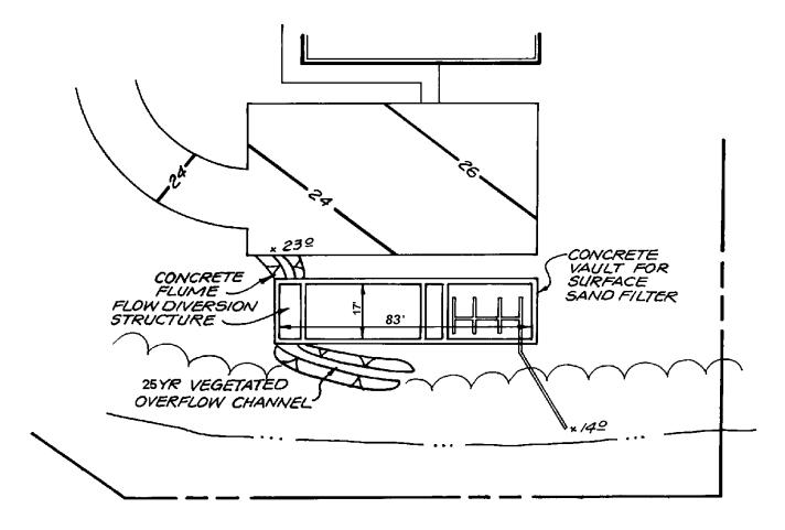
Figure 5. Surface Sand Filter Site Plan
