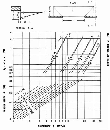
Figure 5.2-9 Depressed Curb-Opening Inlet Capacity in Sump Locations
