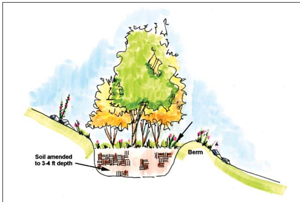
Figure 30. A tree cluster planted on the side slope of a storm water pond helps to treat storm water runoff.
