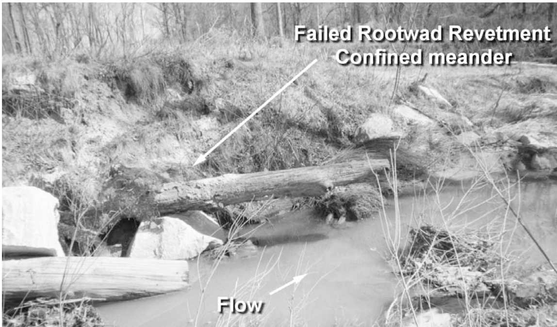
Photo 5.2: Rootwad failure due to channel confinement in meander bend. Lack of access to the floodplain resulted in highly erosive conditions and failure of rootwad revetment.
