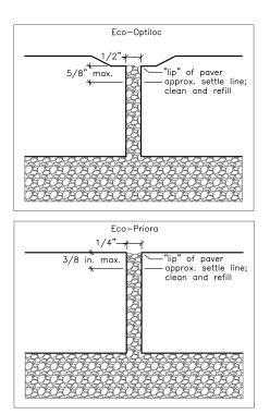
\*Note: Both maintenance types will be most effective when the joint aggregate material is filled to the "lip" of the paver. If the joint material has settled more than the joint width, plus 1/8 inch below the paver lip, the maintenance equipment is significantly less effective and potentially more expensive.
