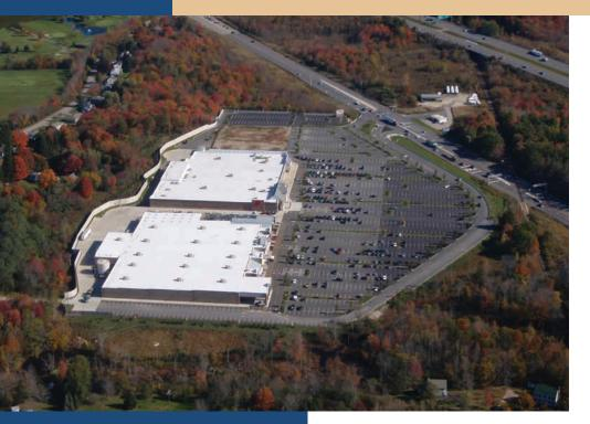
Utilizing an LID approach that featured porous asphalt and a gravel wetland, a cost-competitive drainage system was designed for a large retail development.
