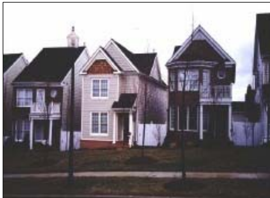
Figure 5. 27 Taller houses create a smaller impervious footprint (Source: Center for Watershed Protection, 2005)
