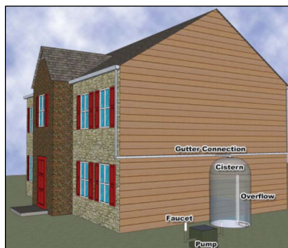
Figure 7.42: Major Components of a Rainwater Harvesting System
