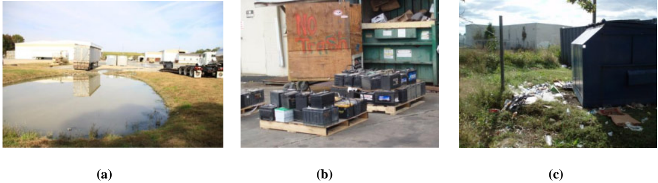
Figure 4. 16. (a) Municipal vehicle washing on impervious surface (TT_HSI_67); (b) batteries stored outside without cover or containment (TT_HSI_22b); and (c) poor trash management (TT_HSI_22a)
