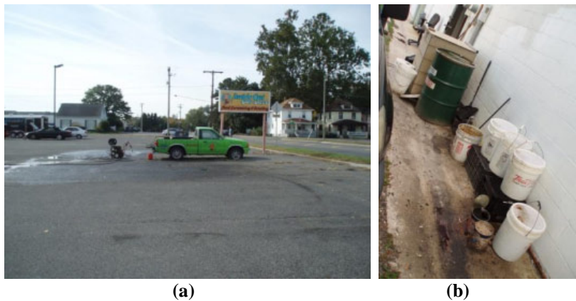
Figure 4. 8. (a) Commercial vehicle washing on impervious cover (HSI_20a) and (b) improperly stored materials (HSI_20b)
