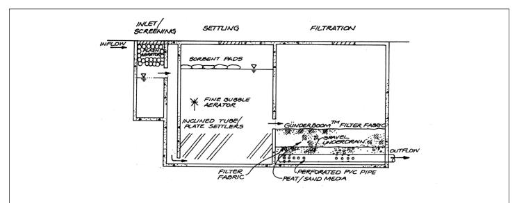
The multi-chamber treatment train (MCTT) consists of three treatment units in sequence—an inlet screening chamber, a sedimentation chamber and a filtration chamber. Most of the high pollutant removal occurs in the last two chambers.
