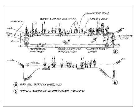
Figure 1: Comparison of Gravel-Based and Surface Stormwater Wetlands
