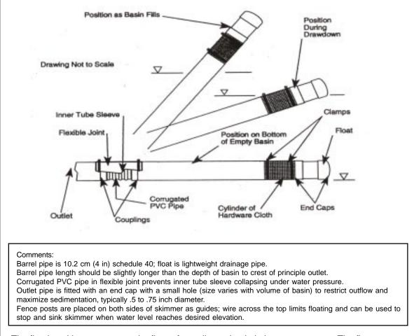
The floating skimmer rests on the floor of a sediment basin in between storms. The float causes the skimmer to rise during a storm, thereby increasing detention time and withdrawing from the less turbid surface waters.
