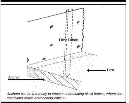
Figure 3: Silt Fence Anchors
