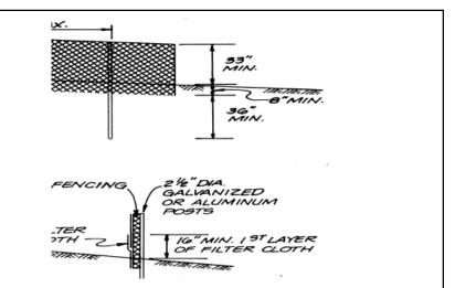
Super silt fence is a useful option in some construction sites where flow lengths or slopes are expected to be too stressful for normal silt fence.
