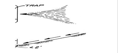
A scoop trap is a practical solution when silt fence is located at the toe of a steep slope.
