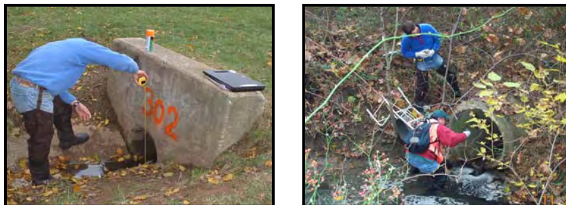
Figure B.4: Discharge investigations will involve more extensive assessments at outfall locations. Local illicit discharge detection and elimination (IDDE) protocols often involve marking outfalls with spray paint and sampling suspected illicit discharges (Brown and Caraco, 2004).
