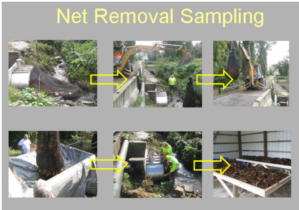
Figure 2. Net removal and transport to drying tables are graphically described. This is Day 1 sampling.
