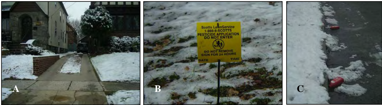
Figure 3-17: Other notable features in residential areas included (A) two-track driveway designs that help reduce impervious cover, (B) evidence of lawn chemical application in the winter, and (C) evidence of homeowner car maintenance with a potential for oil and grease to enter stormdrain.
