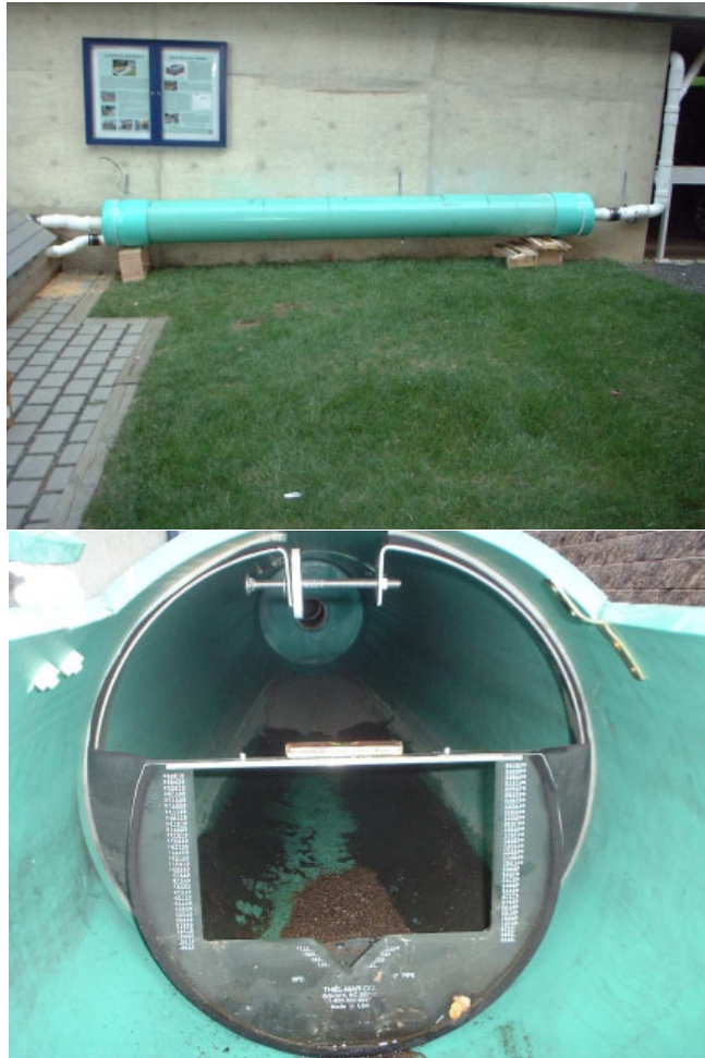
Figure 2-4 a): Installed 15 inch pipe. b): Thel-Mar Weir installed in 15 inch pipe.
