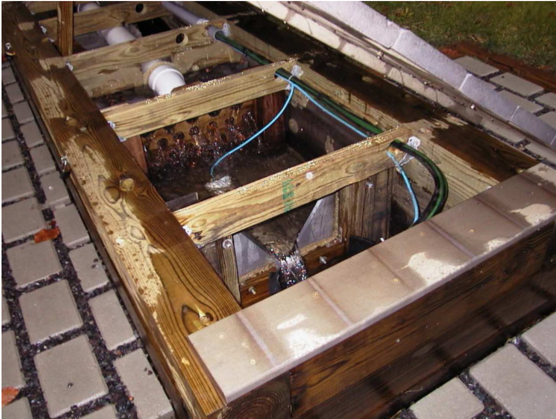
Figure 2-5: V-Notch Weir during a storm event.
