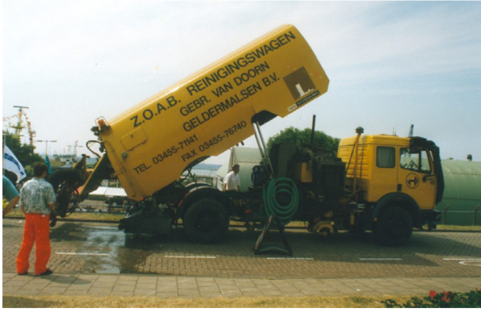
Figure 4.4: PFC (ZOAB in Dutch) cleaning machine.
