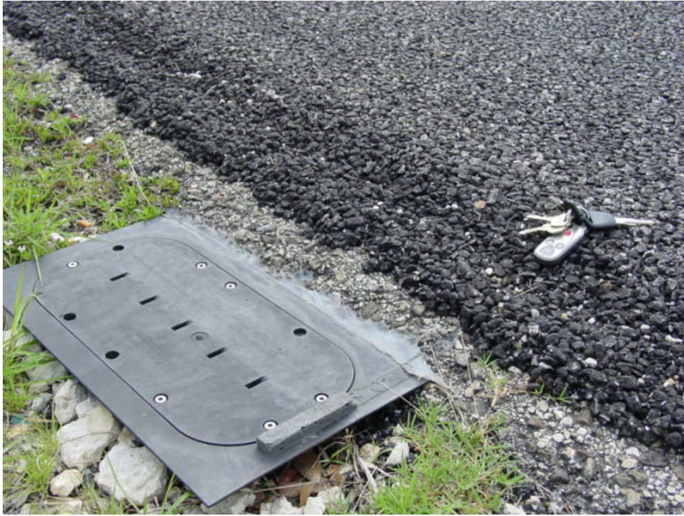
Figure 3.1: Photograph of installed sampler at edge of pavement.
