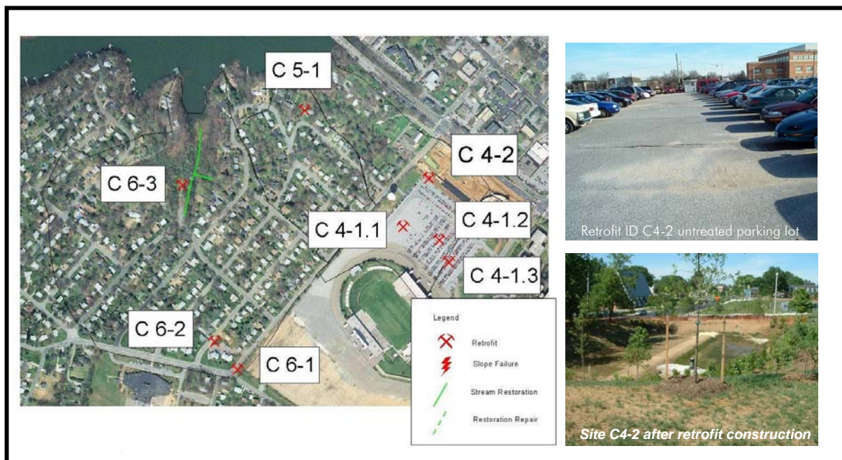
Figure 5.4: Retrofit inventory map (left) and one retrofit example (right) in the Weems Creek watershed in Annapolis, Maryland.
