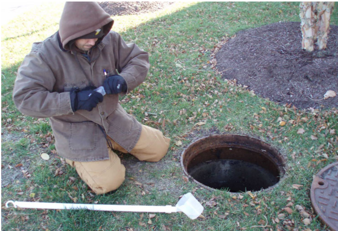
Figure 3.4. Tracking the source of a sewage discharge involves sampling “up the pipe” at manholes to isolate the source of contamination.
