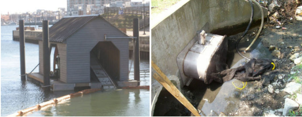
Figure 4.8. The Water Wheel formerly located at mouth of Jones Falls in Baltimore City funnels trash onto a conveyor belt (Sources: Baltimore City Department of Public Works, Talbot County Department of Public Works)
