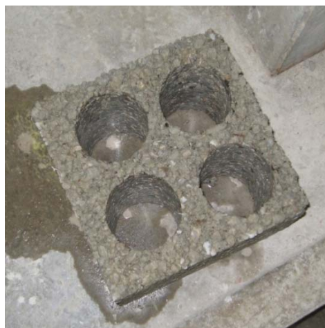
Figure 27. Cores extracted from slabs for material characterization.
