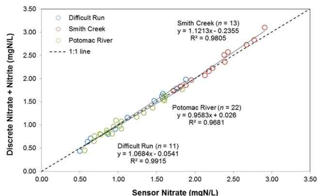
**Figure 2.** Relationship between nitrate concentrations measured in the laboratory from discrete water quality samples and concentrations measured by the in situ sensors at Potomac River, Smith Creek, and Difficult Run.
