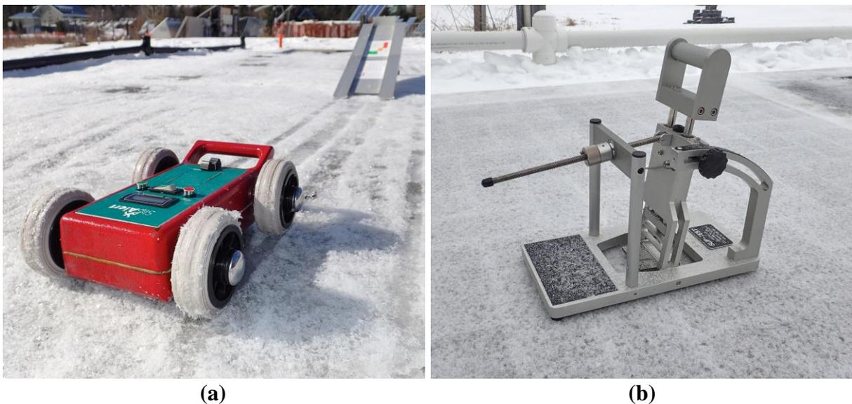
**Figure 3: Surface friction measuring devices in use on ice covered PICP surfaces: (a) SlipAlert and (b) Mark IIIB.**
