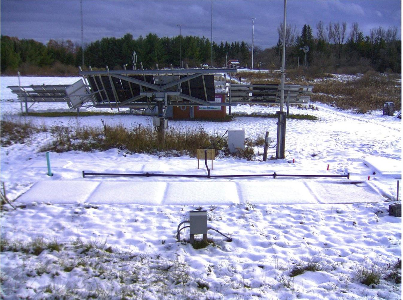
**Figure A3: Snow cover conditions on 17/Nov/2018 where mounds formed on pervious surfaces (PICP cells and catch basin) after snow structures collapsed during slow melting processes on the surrounding impervious surfaces (asphalt cell and concrete barriers).**
