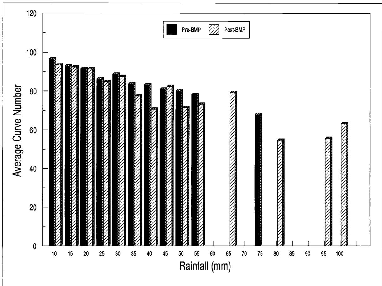
Figure 3. Variations of Watershed-Averaged Curve Number with Storms for the Pre- and Post-BMP Periods.
