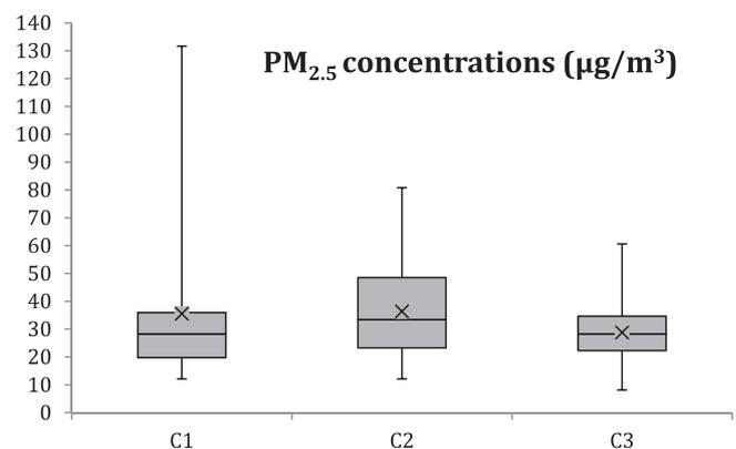
Fig. 3. Box and whisker plot of PM<sub>2.5</sub> concentrations for the three cases; mean (cross sign), median (solid line in box), 25th and 75th percentiles (upper and lower ends of boxes), 10th and 90th percentiles (upper and lower whiskers).
