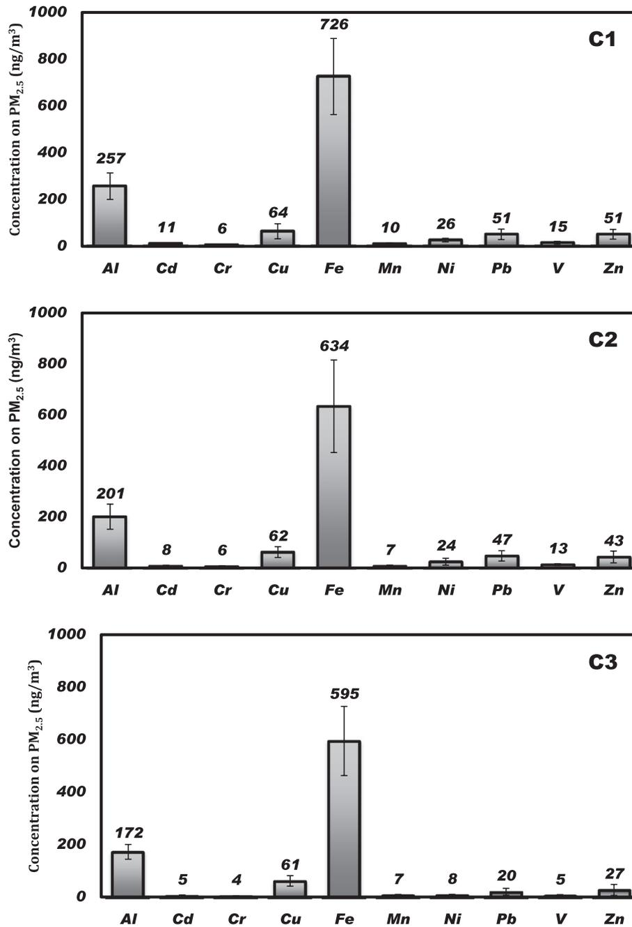
Fig. 5. Concentrations of HMs (ng m<sup>-3</sup>) in PM<sub>2.5</sub> (values above the bars show the mean values).
