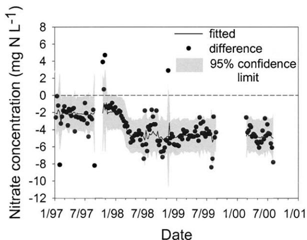
Fig. 5. Nitrate concentrations in the treated subbasin (TR1) minus concentrations in the control subbasin (CN2) during the late spring nitrate test (LSNT) treatment period and the fitted quadratic model with a Lag 1 residual component at its 95% confidence limits. Concentrations from the two subbasins are significantly different when the confidence limits do not include the 0 difference line.
