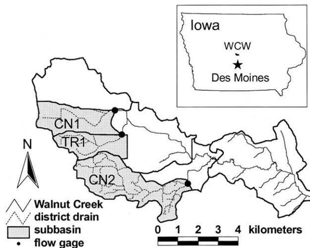
Fig. 1. Location of Walnut Creek watershed (WCW) within the state of Iowa (inset), and the location of the stream, district drains, discharge gaging stations, control subbasins (CN1 and CN2), and treatment subbasin (TR1) within WCW.
