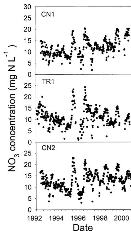
**Fig. 3. Nitrate concentration in drainage from the control (CN1 and CN2) and treated (TR1) subbasins.**
