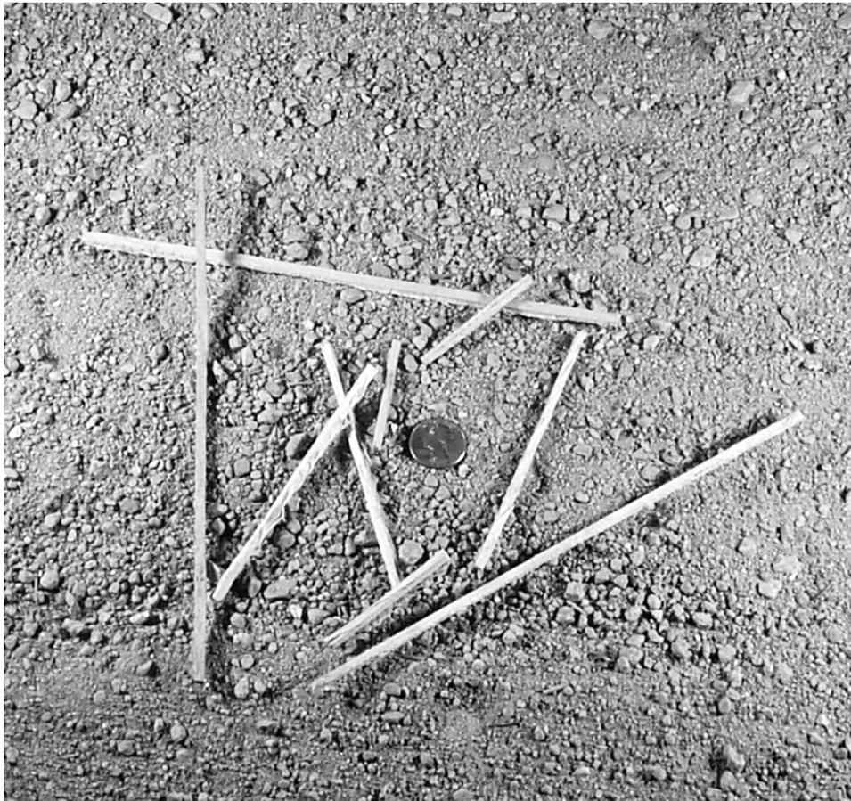
**Figure 2.** Narrow strands on soil used in this study. Longest strands are 240 mm long, intermediate strands are 120 mm, and shortest strands are 60 mm. All are 4 mm wide and 3 to 4 mm thick. Note the quarter for scale.
