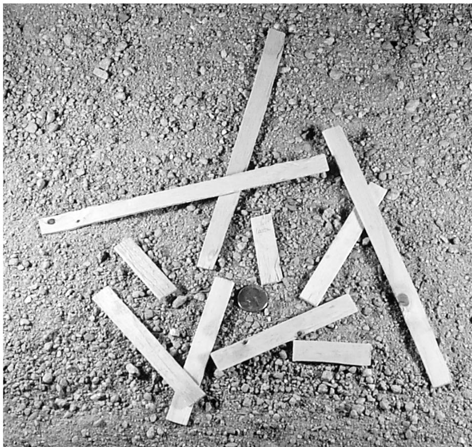
**Figure 1.** Wide strands on soil used in this study. Longest strands are 240 mm, intermediate strands are 120 mm, and shortest strands are 60 mm. All are 16 mm wide and 3 to 4 mm thick. Note the quarter for scale.
