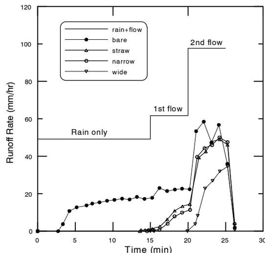
Figure 4. Average runoff hydrographs for each treatment.
