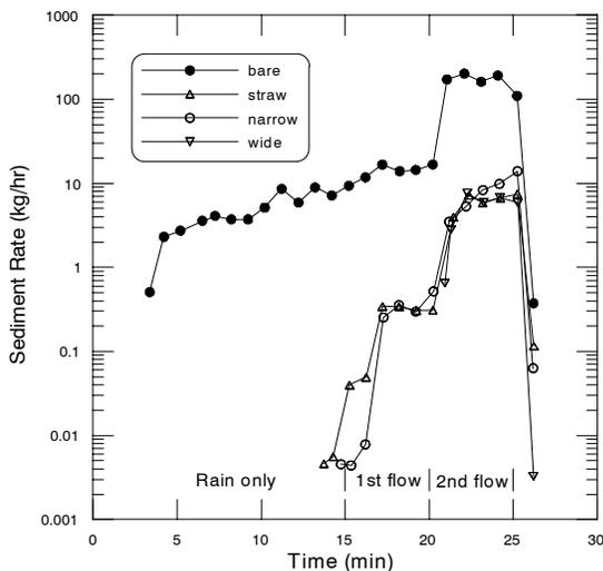
**Figure 5. Average sediment rate for each treatment. Note the logarithmic scale of the sediment rate.**
