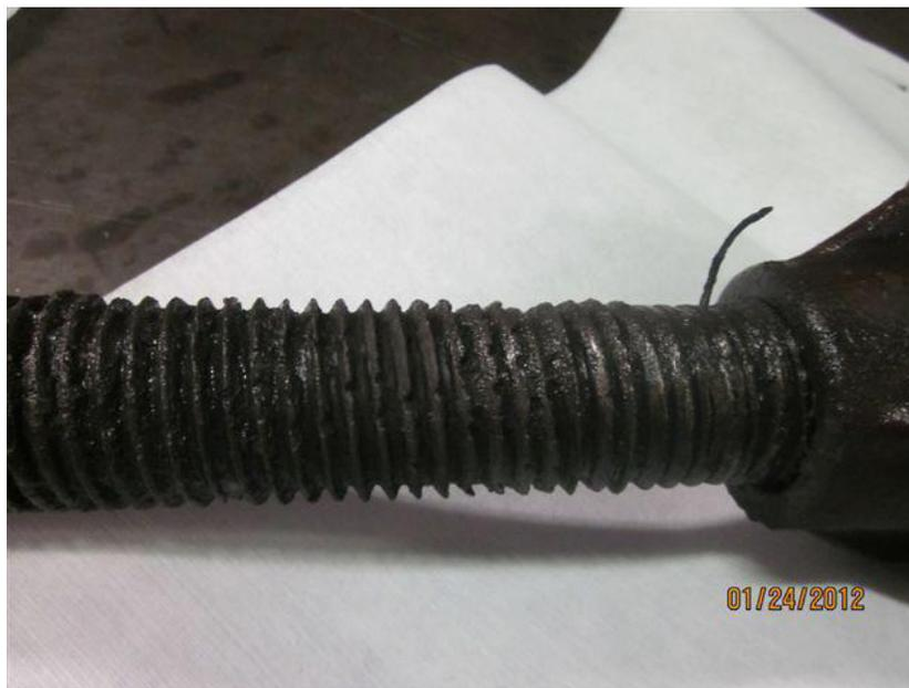
FIGURE 6.13. CORRODED LANDING LEG SCREW (PHOTO FROM [126])
