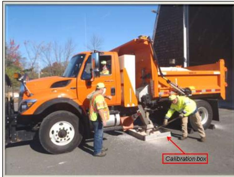
Figure 13: Spreader calibration
