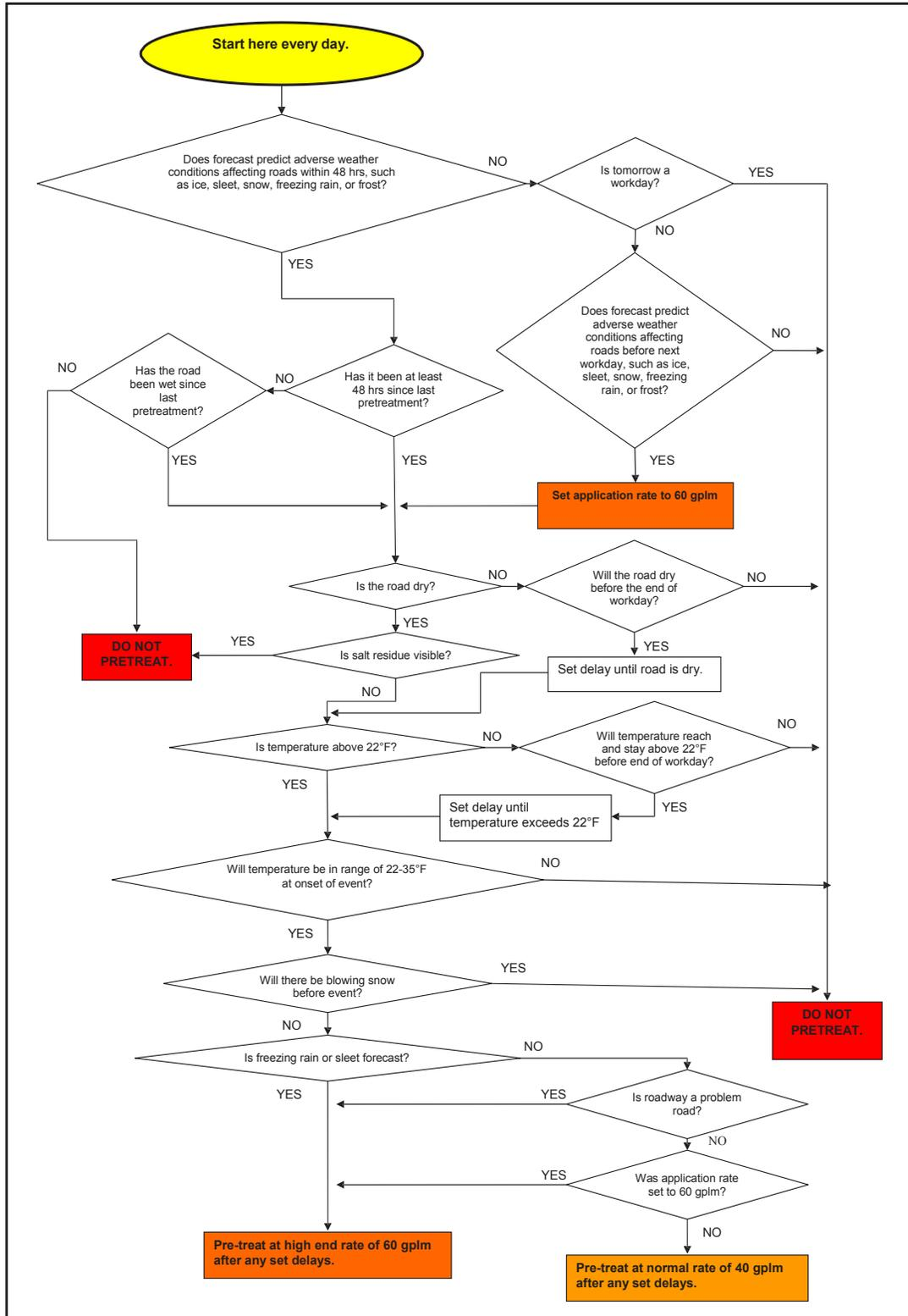
Figure 4: Decision Flowchart for Pre-Treatment in Connecticut
