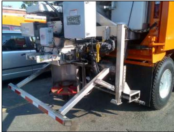
Figure 17: Salt-Slurry Generator
