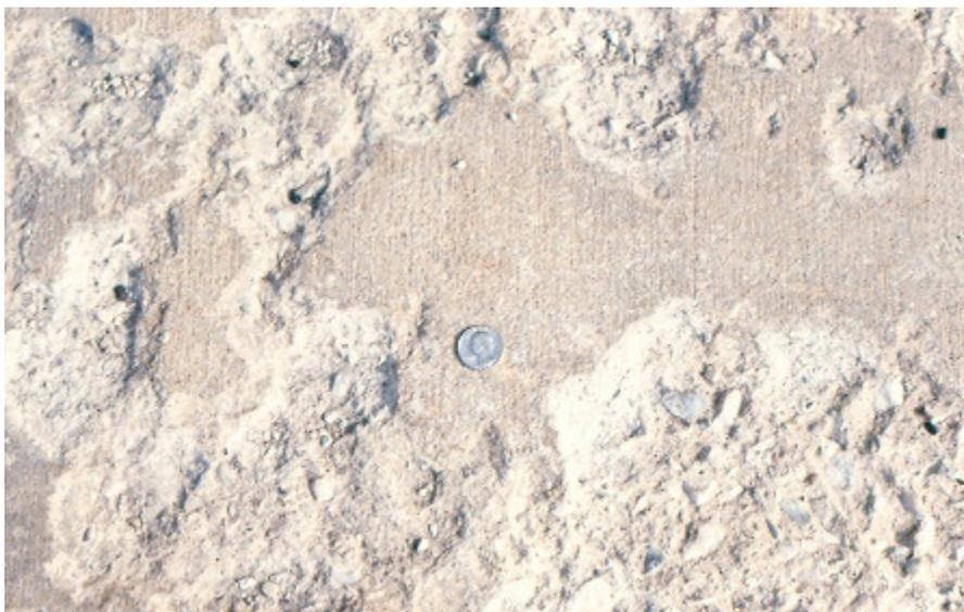
FIGURE 6.4. PORTLAND CEMENT CONCRETE SURFACE SCALING (PHOTO FROM [92])
