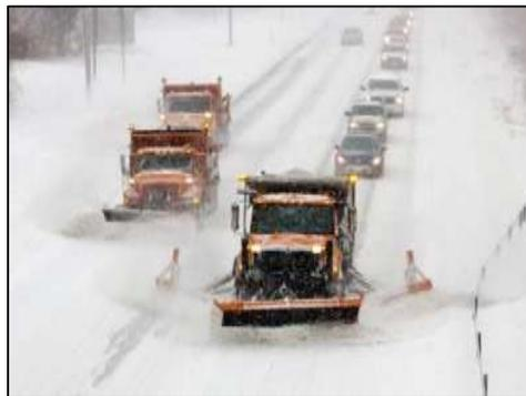
Figure 10: Trucks Deployed in Echelon
