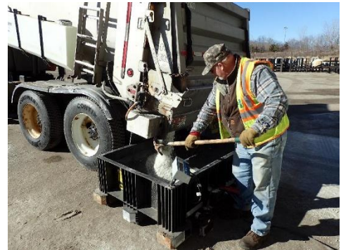
Above, an operator is performing a catch test with a scale box.
