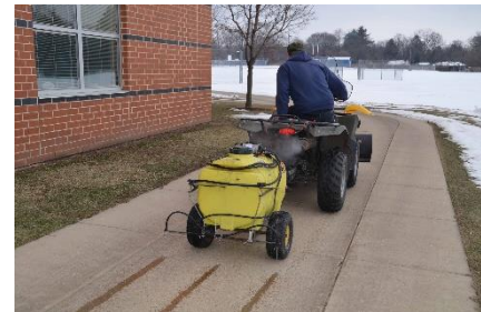
Above an ATV is applying deicer in a wet/dry spread pattern
