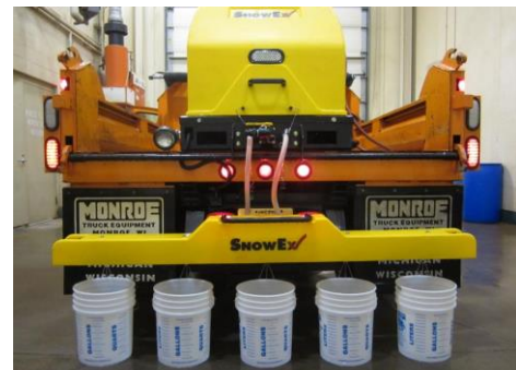
Individual catch test buckets give nozzle discharge plus total discharge
