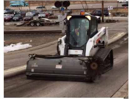
This photo shows one example of equipment used for sand sweeping.
