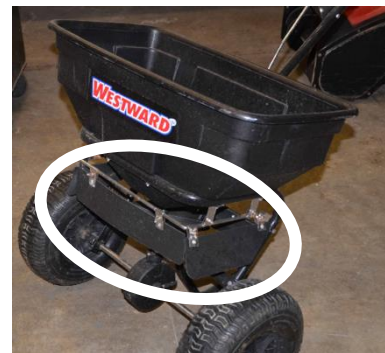
Example of a shield for a spreader to create a narrower spread pattern
