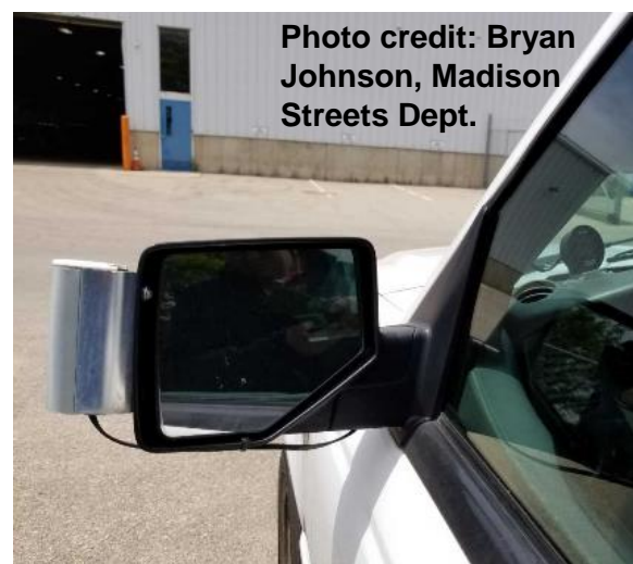
Mirror-mounted temperature sensor
