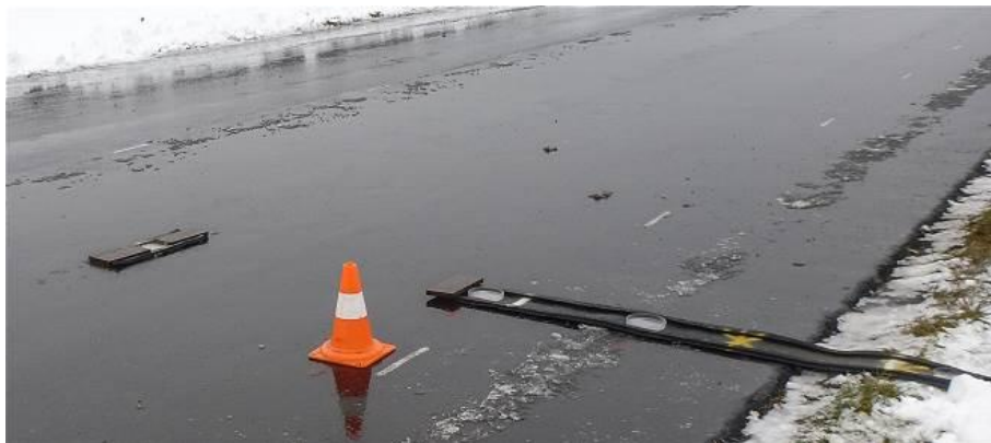
Figure 8 – Sampling the salt deposition (new pavement).
