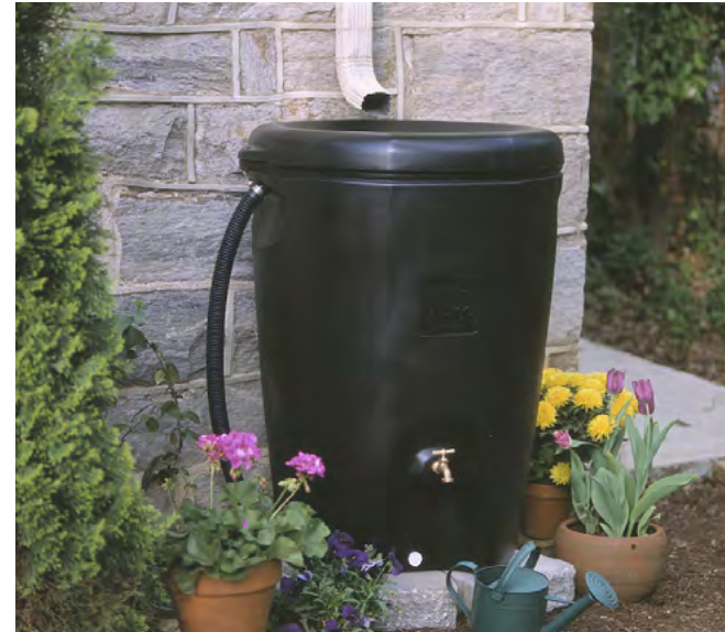
A disconnected downspout and rain barrel. Photo: Clean Air Gardening
