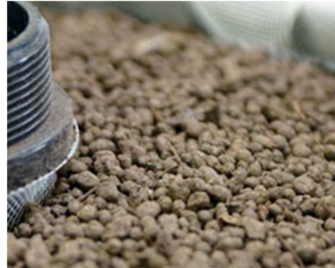
Media filter media can be customized to target specific pollutants. Photo: Contech
