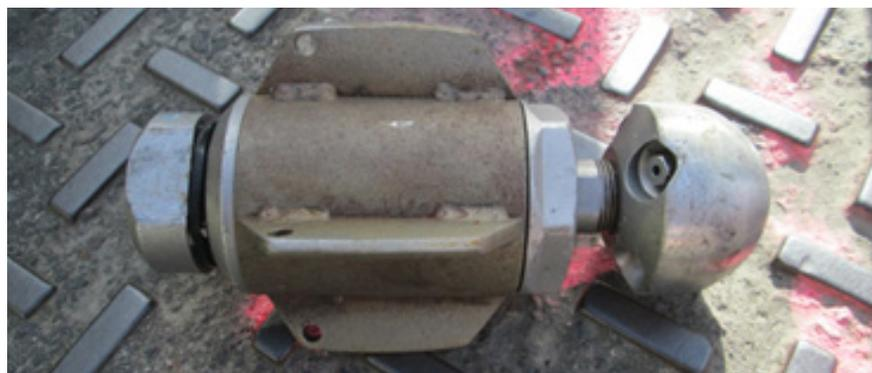
Figure 3-6. Rotating nozzle with three rear-facing jet-rods and rotating center
