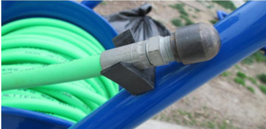
Figure 3-1. Small flushing nozzle
