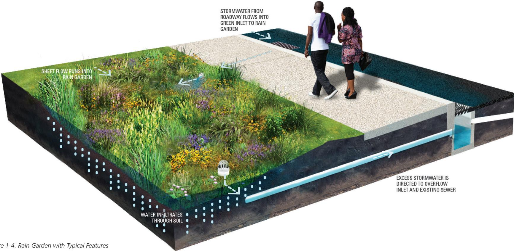
Figure 1-4. Rain Garden with Typical Features
