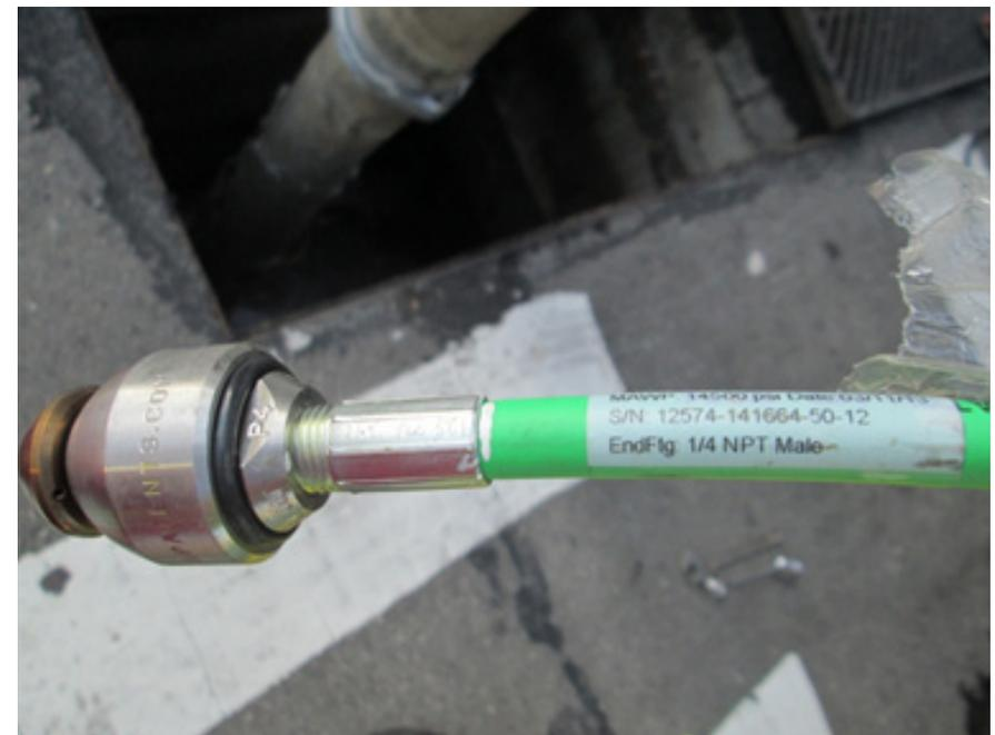
Figure 3-7: Small rotating, root cutting nozzle
