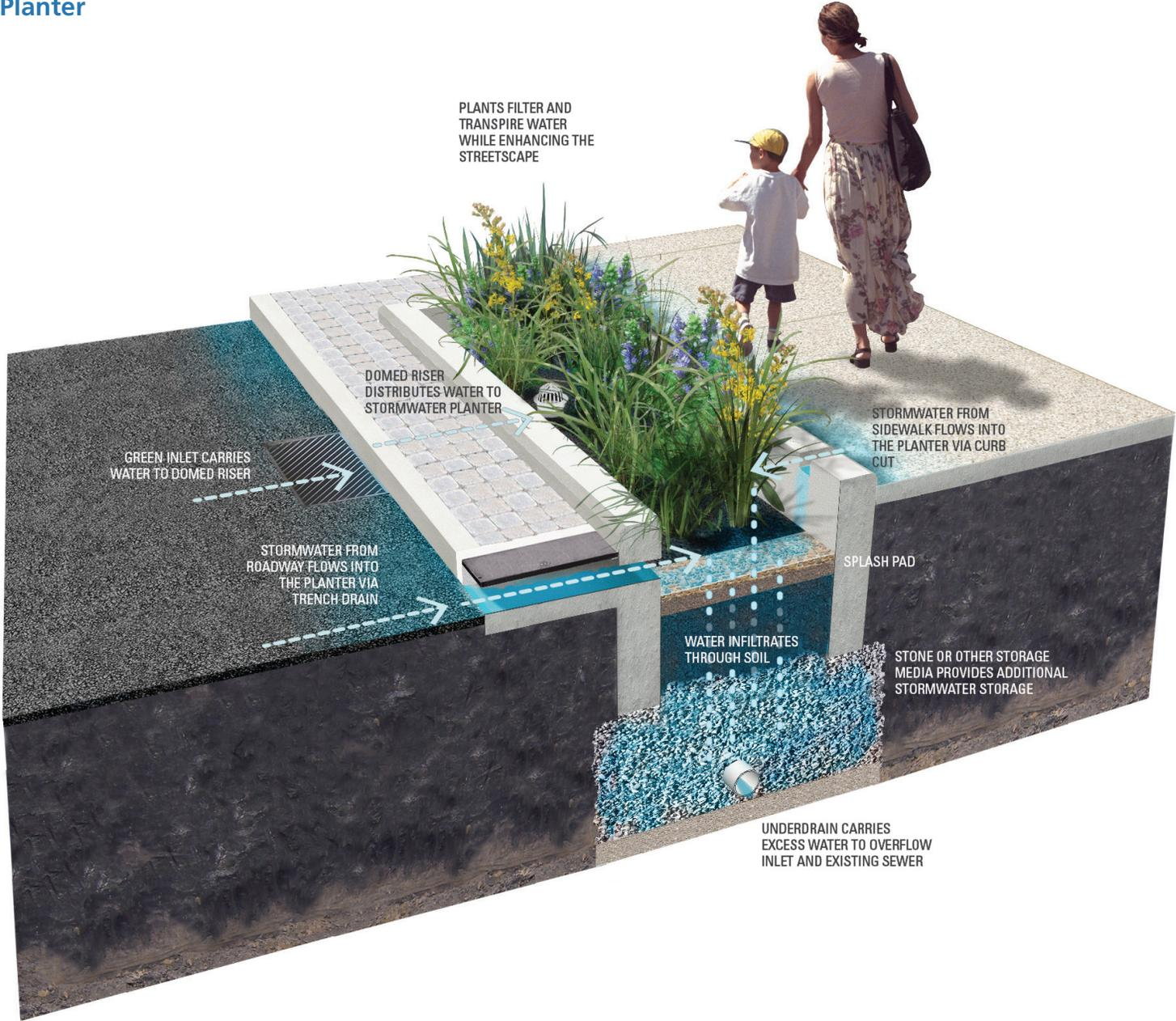
Figure 1-6. Stormwater Planter Section Typical Features
