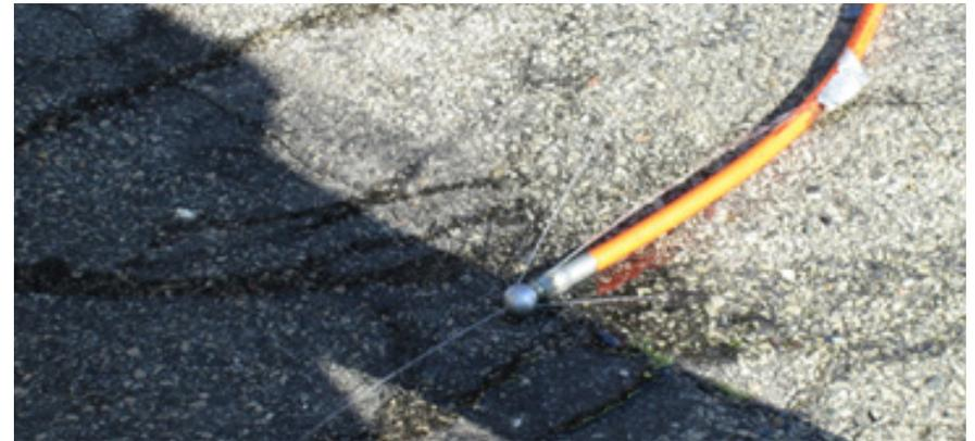
Figure 3-3. Small penetrating nozzle with one front facing and six rear-facing jet-rods
