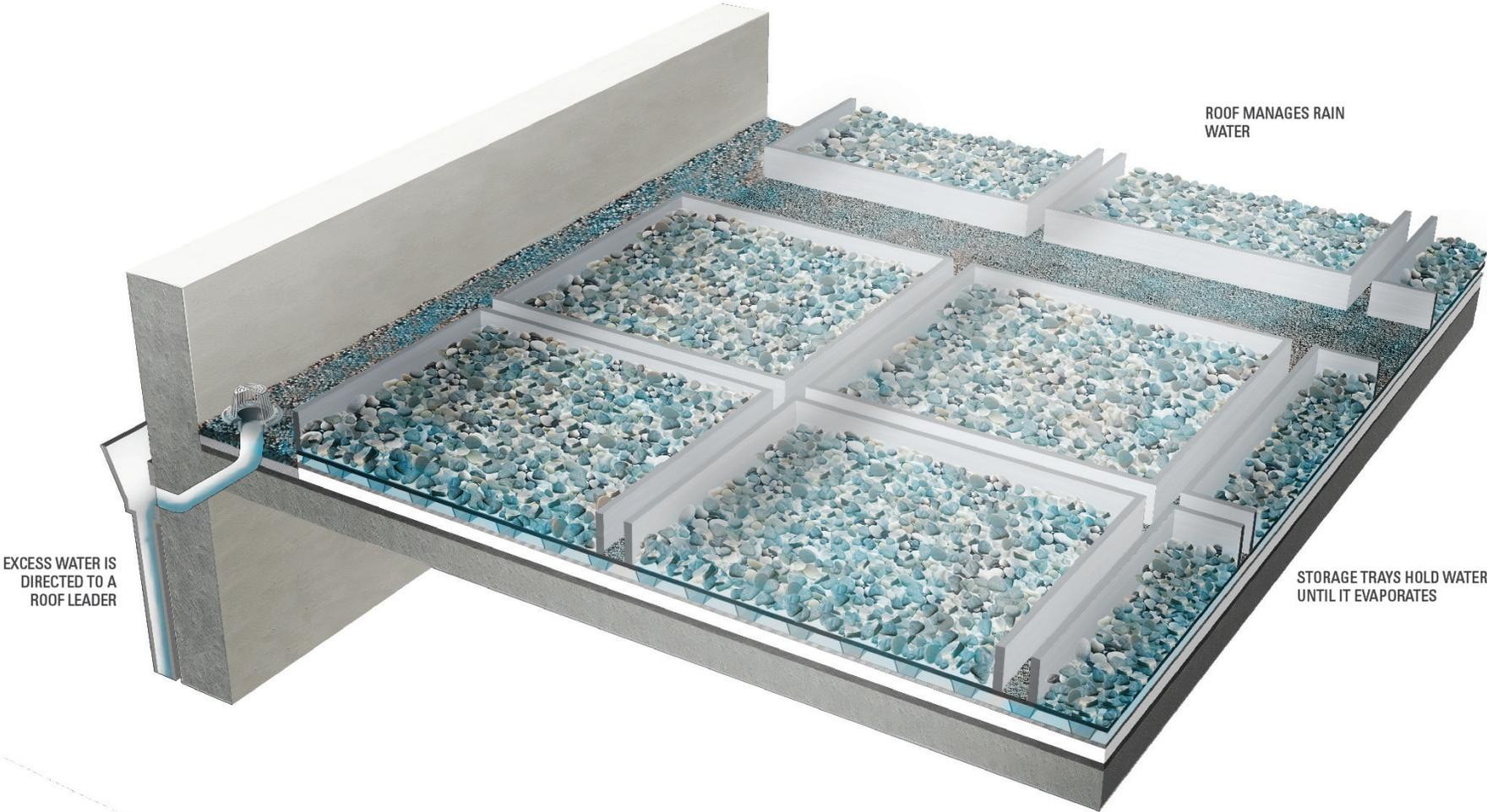
Figure 1-27. Blue Roof Detention Tray, Check Dam, and Modified Roof Leader System
