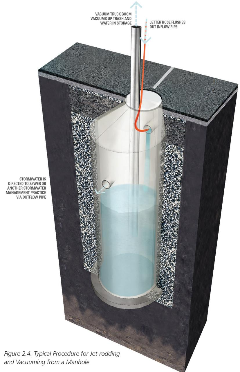
Figure 2.4. Typical Procedure for Jet-rodding and Vacuuming from a Manhole
