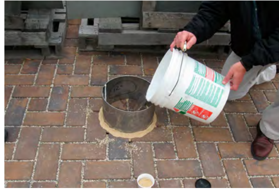
Figure 8-8 Inexpensive test apparatus for implementing ASTM C1701 and C1781 methods for assessing surface infiltration rates and cleaning needs for permeable pavements (PICP shown here) Source: Interlocking Concrete Pavement Institute (ICPI)
