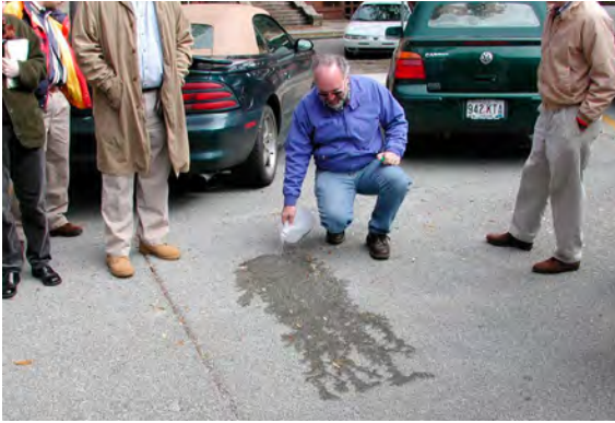
Figure 8-7 Demonstration of clogged pervious concrete surface using one gallon of water, Savannah, Georgia Source: NCSU
