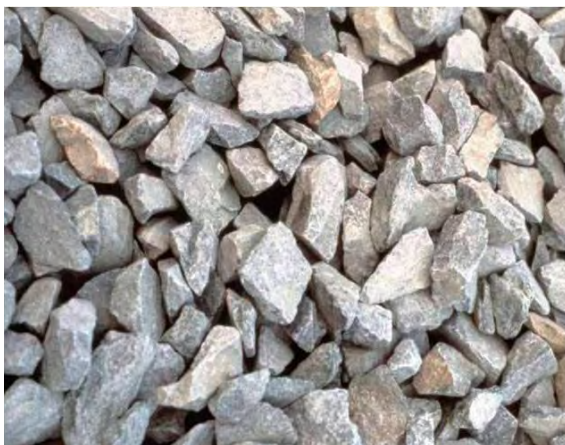
Figure 2-18 Clean, washed, crushed storage bed aggregate
