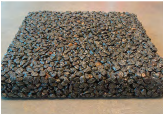
Figure 6-1 Example of a pervious paver bound with a polymer Xeripave® Source: CH2M HILL
