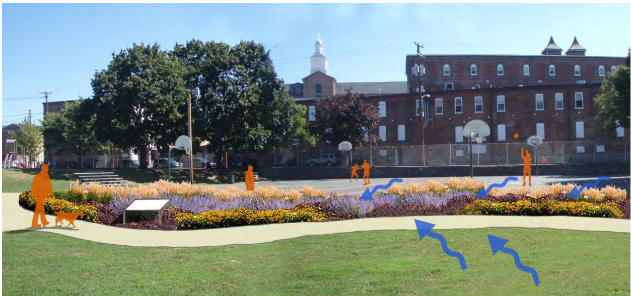
Bioretention manages runoff from basketball court (Rendering - TCA, Inc., 2010)
