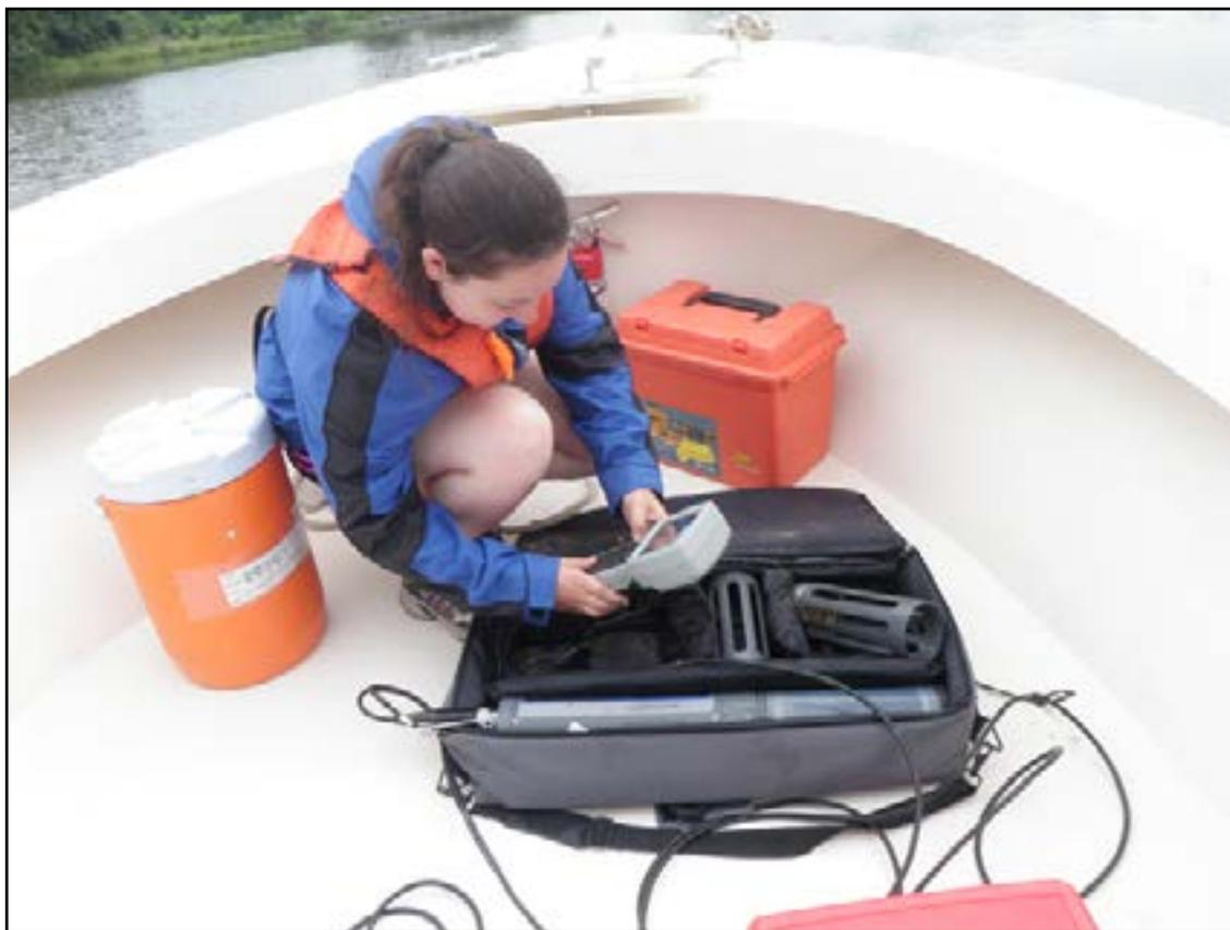
**Image WQ2.** A YSI data sonde® (YSI, Inc., Yellow Springs, OH) is being assembled prior to measuring water quality parameters such as dissolved oxygen, temperature, salinity, and turbidity in the Tred Avon River ecological assessment.
