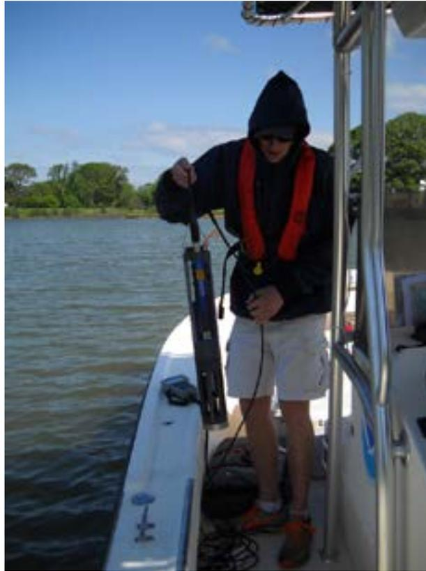
**Image WQ3.** A YSI data sonde® (YSI, Inc., Yellow Springs, OH) is used to measure water quality parameters in the Tred Avon ecological assessment.
