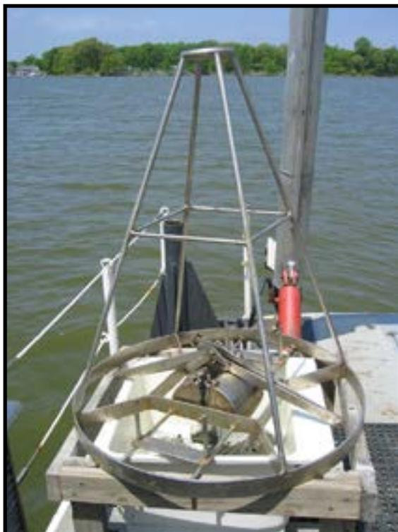
**Image BH1.** A Young-modified Van Veen grab is used to collect sediments for laboratory analyses.
