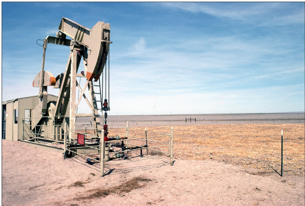
Figure 26 —Pumpjack for an oil well, Pawnee National Grassland, Colorado (source: USDA Forest Service, https://www.fs.usda.gov/detailfull/arp/home/?cid=STELPRDB5356427&width=full ).
