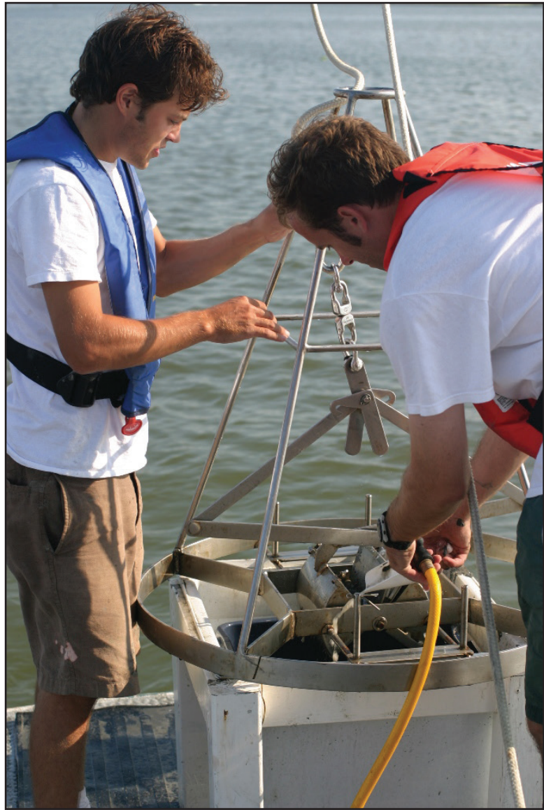
Scientists deploy a Young modified Van Veen benthic grab sampler to collect benthic community and sediment samples.
