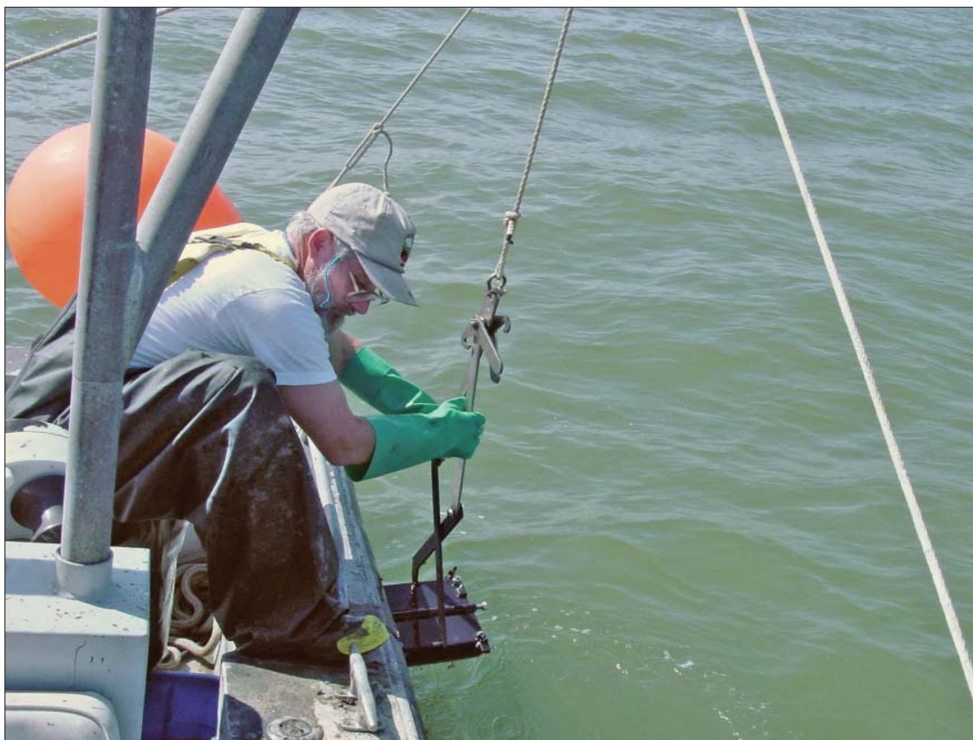
Researcher collects samples of sediment and benthic infauna in the Chesapeake Bay. Photo credit: NOAA CCMA COAST
