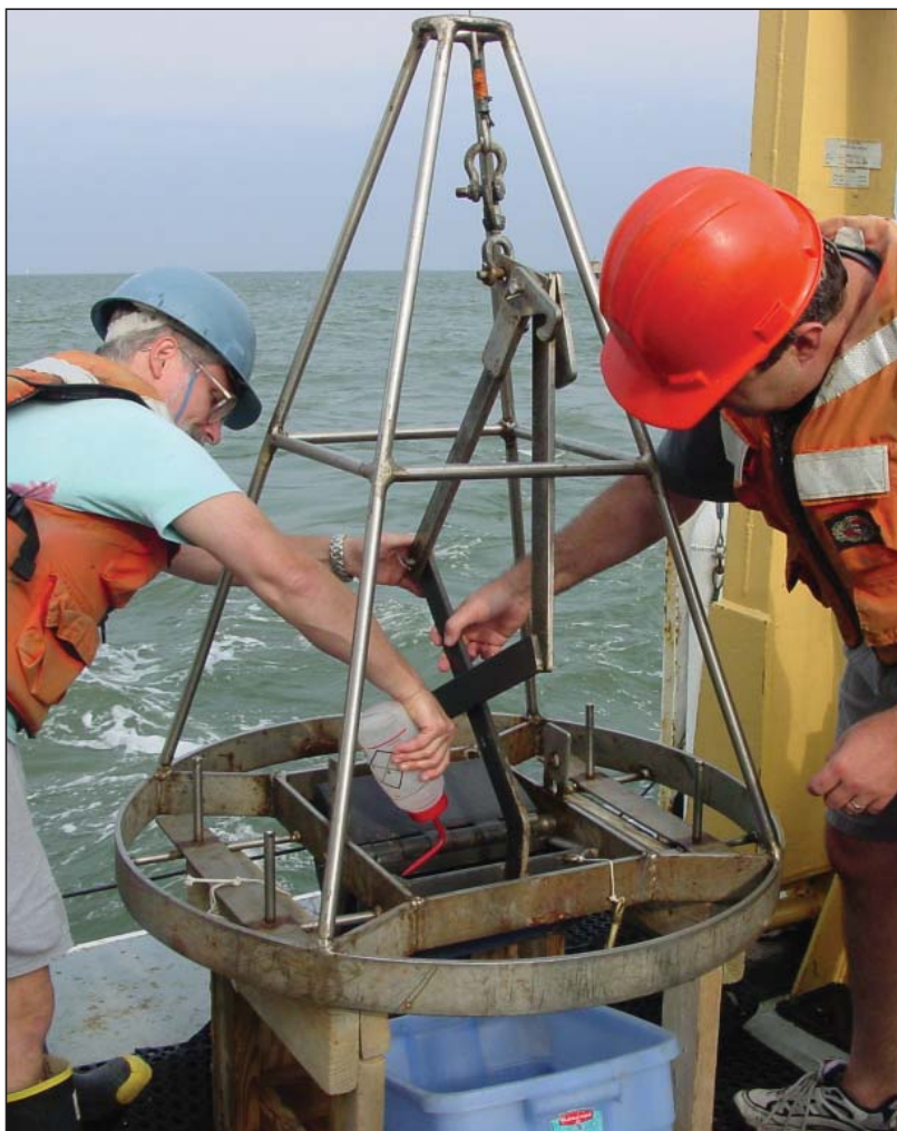
Scientists prepare the Young Grab for sampling. Photo credit: NOAA CCMA COAST
