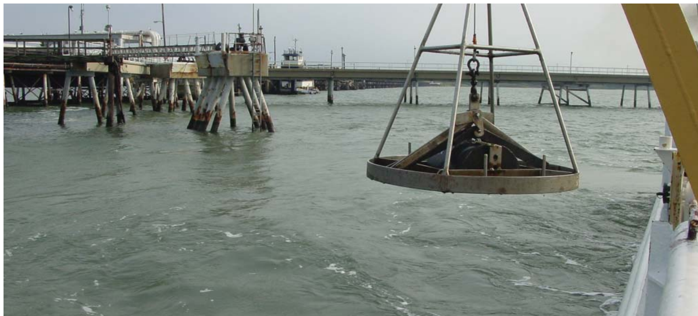
Young Grab being deployed for sampling. Photo credit: NOAA CCMA COAST
