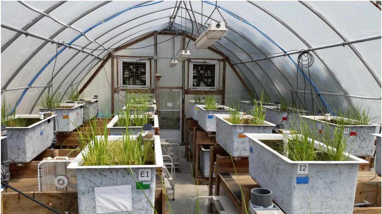
**Figure 1.** Individual mesocosm test systems enclosed in the greenhouse, NCCOS laboratory, Charleston SC.
