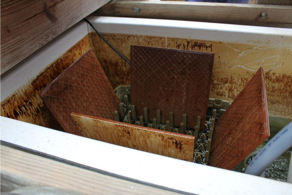
**Figure 3.** Ceramic tiles after oil was applied to the treatments and one tile was removed to determine mass of oil on the tile.
