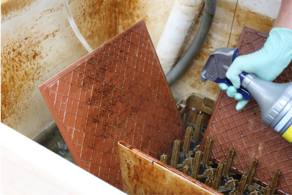
**Figure 4.** Shoreline cleaner product being applied to the oiled tiles.
