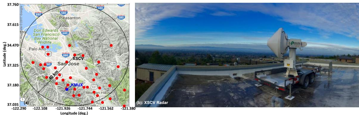
Fig. 5. (a) Location and coverage map of the X-band dual-polarization XSCV radar in Santa Clara, CA; (b) photo of the XSCV radar during the deployment at the SCVWD Penitencia Water Treatment Plant. The coverage range is 40 km. The red dots in (a) denote the locations of rainfall gauges operated by SCVWD. The blue dot in (a) shows the location of the S-band KMUX NEXRAD radar.
